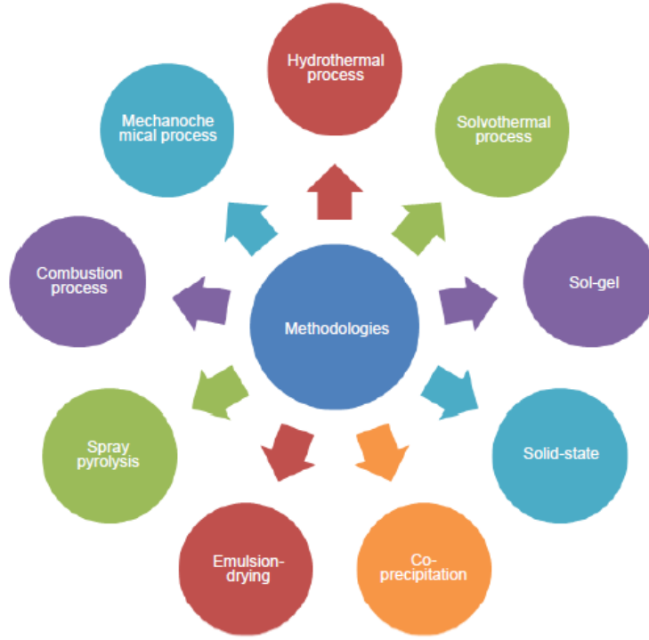
Figure 1.3. Different synthesis techniques utilized to produce cathode materials [26]
