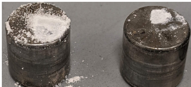
Figure 4.20. An example of a ‘no-go’ after an impact test.
