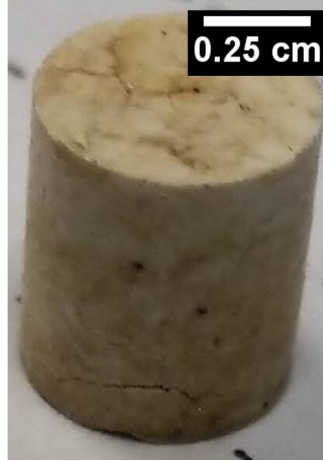
Figure B.1. S-H3 after heating and cooling. No surface cracking was apparent immediately after removal from the oven, however, some surface cracking appeared approximately 24 hours after cooling to room temperature.
