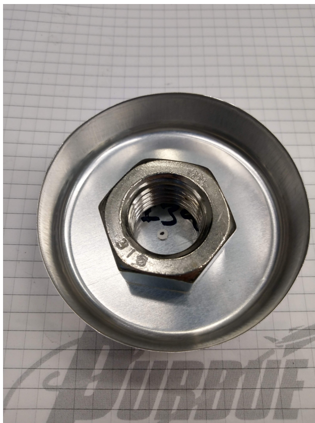
Figure A.3. Aluminum pan with 3 x 1 mm PBX 9501 pellet placed in the center of a weight (used to keep the light-weight pan & pellet from moving due to convection currents within the oven).
