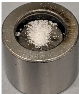
Figure 4.18. An HMX sample placed on a BAM pin surrounded by its collar prior to impact testing. The BAM pin diameter is 10 mm.
