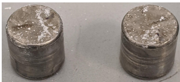
Figure 4.19. An example of a ‘go’ after an impact test.
