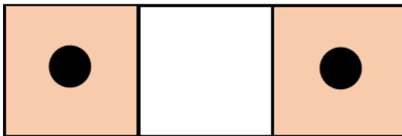
Figure 1.4. A three-choice housing system for preference testing in piglets, as described by Vasdal et al., (2010). The apparatus includes two thermal compartments (left and right) with infrared heating lamps located above (black circles) to control temperature within each compartment. The middle compartment was a neutral compartment that was 2-20°C cooler than either thermal compartment. Temperatures were altered such that piglets experienced a combination of: 26°C vs. 34°C, 26°C vs. 42°C, or 34°C vs. 42°C.
