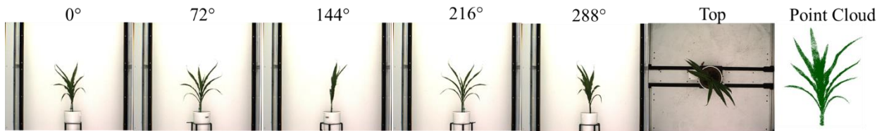
Figure 3.4. Overlapped images acquired for generating point clouds
