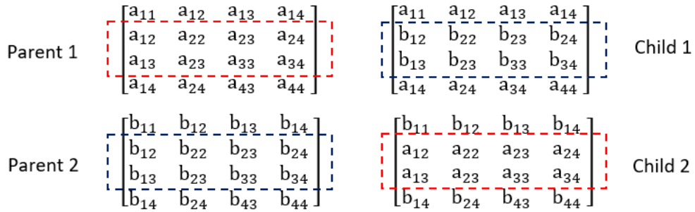
Figure 1.6. Illustration of the crossover variant-4 that mixes the SNN weights of two bots for the “Crossover and Mutation” strategy described in Section 1.3.7. While the illustration is with 4 \times 4 matrices, the SNN weight matrices are 30 \times 30 .
