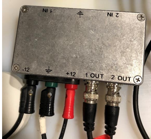
Figure 3.4 This is the updated, enclosed version of the voltage follower with better streamlining of inputs and outputs. This final version was the one used during all of the anesthetized and awake experiments.
