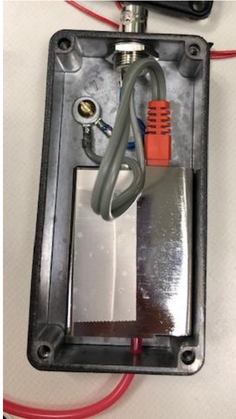
Figure 3.1 Example of the acoustic transducers in the electrically shielded boxes. The transducer is wrapped in shielding tape and is grounded to the box.
