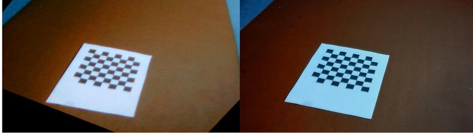
**Figure 7.4.** Reprojection of camera 2 image to camera 1 image using homography matrix.
