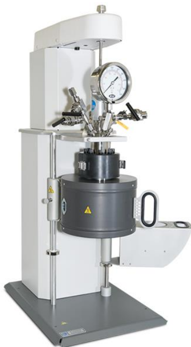
Figure 3. 2 Parr type 4570 high-temperature high-pressure batch reactor ( www.parrinst.com )
