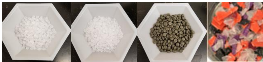
Figure 3. 1 Standard PP polymer pellets, standard PE polymer pellets, pelletized PE waste, and shredded PP waste (from left to right)
