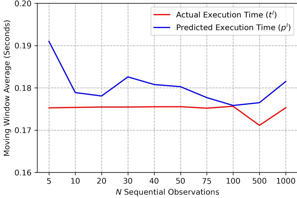
Figure 5.6. Running window mean for cloud actual execution time ( t^l ) and predicted time ( p^l ). Maximum prediction accuracy is achieved at around N = 100 .
