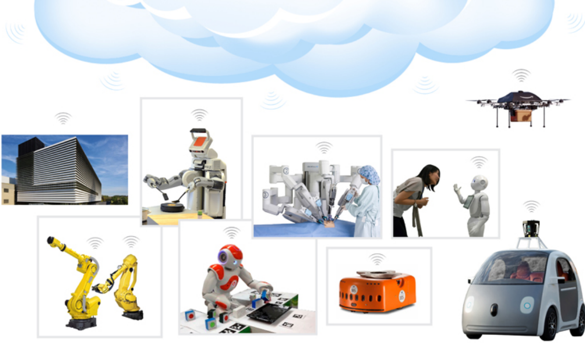
Figure 1.1. Generic cloud robotic architecture showing robots connected to cloud computing through wireless network. [4][© 2015 IEEE].
