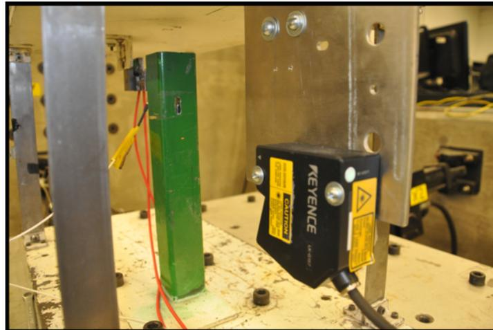
Figure 4.16. Keyence Laser Sensor
