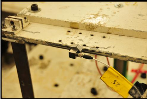
Figure 4.14. PCB Accelerometer
