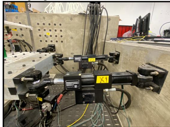
Figure 4.19. Hydraulic Actuators
