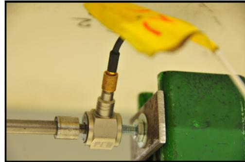
Figure 4.15. PCB Force Sensor
