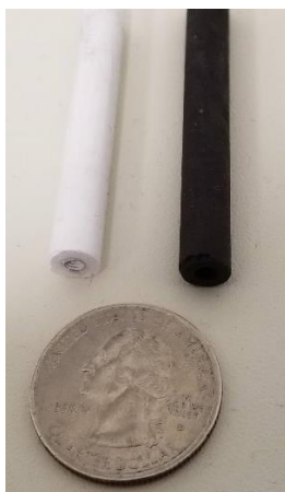
Figure 5. Composite samples containing (left) barium strontium titanate (BST) and (right) nickel zinc ferrite (NZF) inclusions. The quarter is included for scale.
