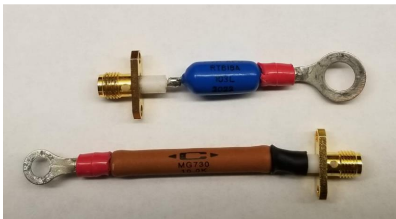
Figure A- 1. High voltage resistors used in voltage divider (top) HVR RT series and (bottom) Caddock MG730 series. Both resistors have a 10 k \Omega resistance.
