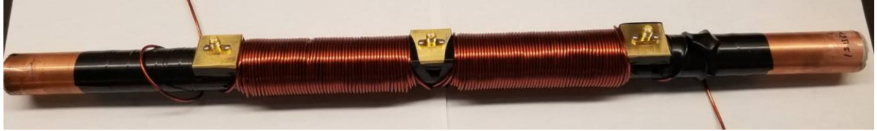
Figure 28. Final NLTL after winding 14 AWG magnet wire around line for bias. The three brass connectors are D-dot probes to assess the wave propagation through the line.
