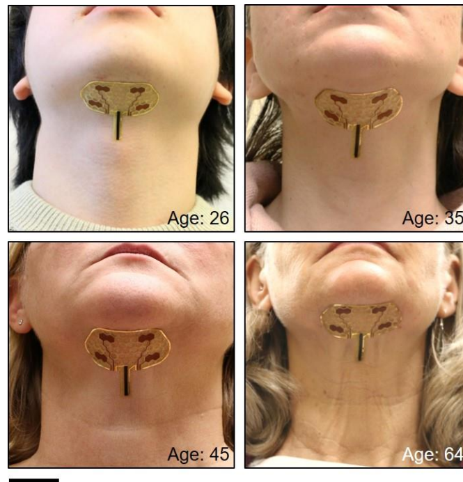
Figure 2.2. Sensor patch adhered to the submental area of subjects of different ages. Photos of the sensor patch placed on human subjects of different ages (26~64).
