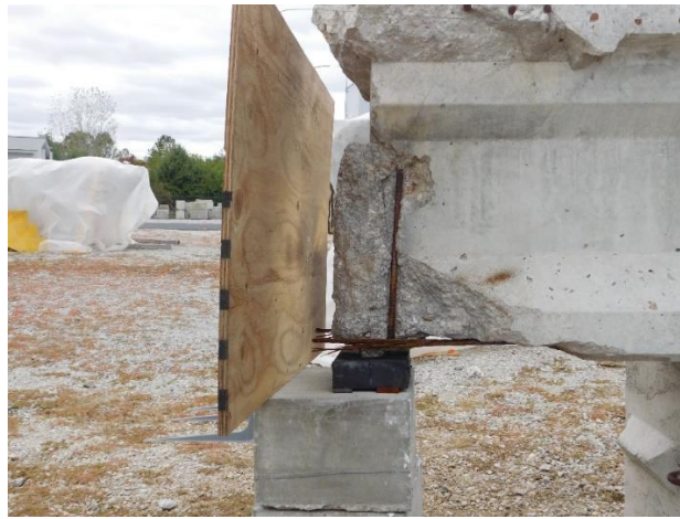
Figure 3.24 Simulated Mud Wall and Bearing Pad Location for NSM FRP Specimen
