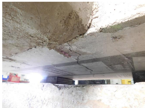
(b) Bottom Surface of Diaphragm at Shear Force of 44 Kips
