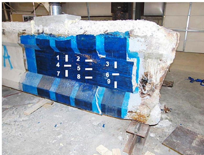
Figure 2.14 CFRP Repair System with Vertical U-Wrap and Longitudinal Strip Anchorage (from Petty et. al 2011)
