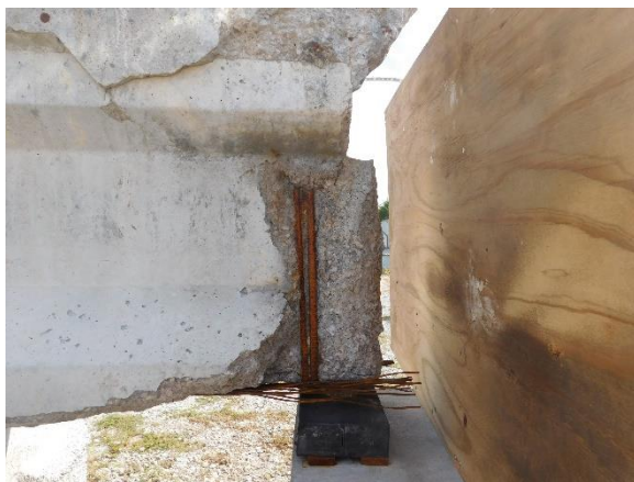
(c) Condition After Sandblasting
