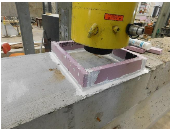
(a) Closed-Cell Polystyrene Formwork
