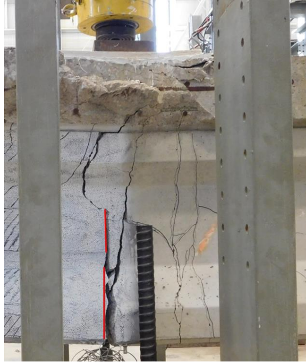
Figure 4.13 Critical Flexural Crack of Externally Bonded FRP Specimen After Failure
