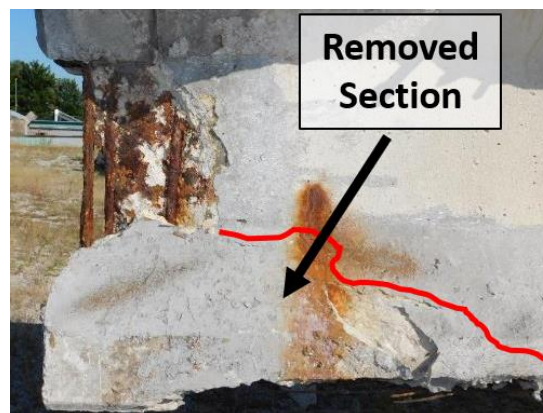
Figure 3.27 Flange Portion Removed from Supplement Diaphragm Specimen
