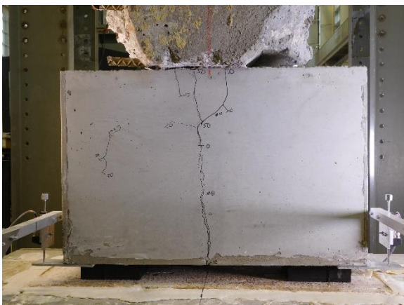
(a) End Face of Diaphragm at Shear Force of 44 Kips
