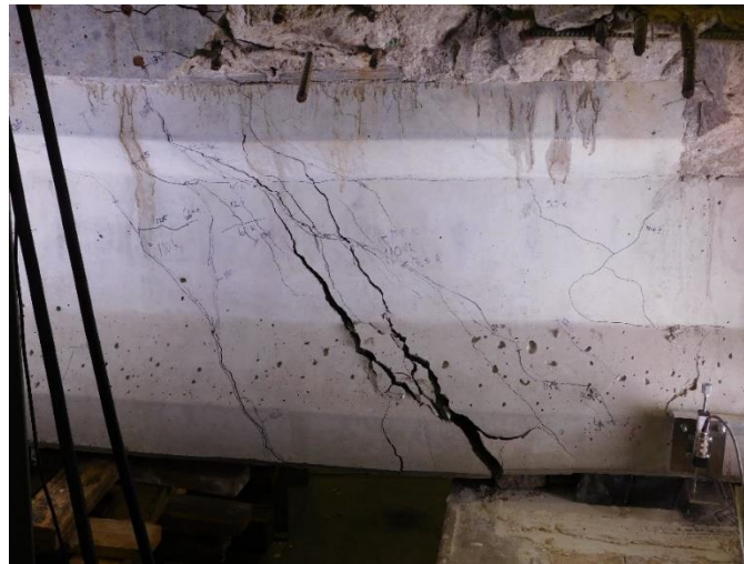
Figure 3.6 Control Specimen After Failure
