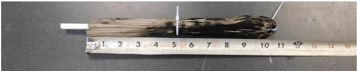
Figure 3.23 Assembled FRP Spike Anchor for Bottom Flange Installation
