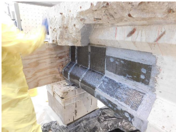
(f) Externally Bonded Strips/Sheets Applied to Specimen
