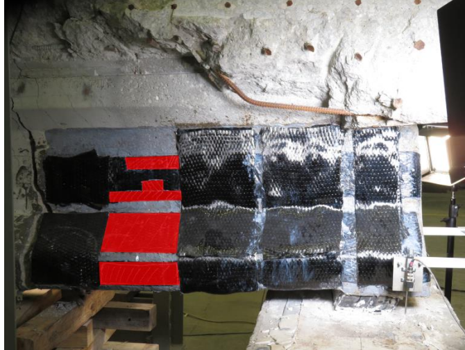
Figure 4.11 Externally Bonded FRP Specimen After Failure
