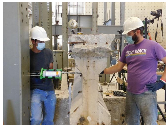
(b) Injecting Hole with Epoxy
