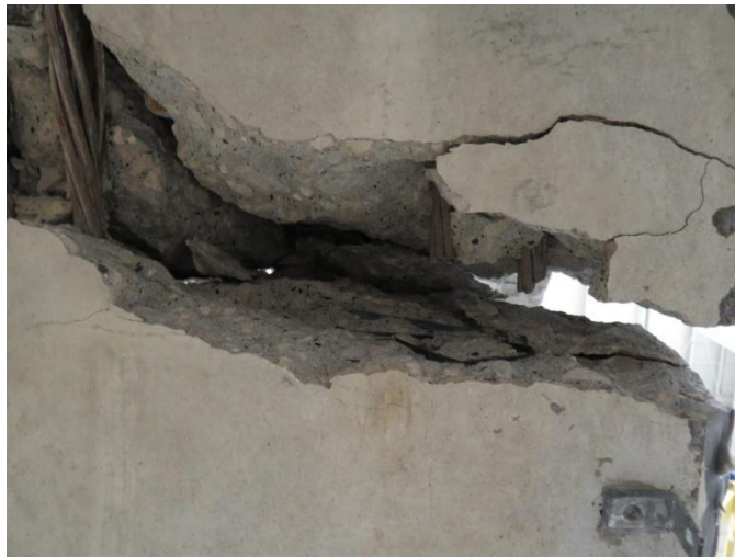
Figure 4.12 Fractured Prestressing Strands in Bottom Flange After Testing
