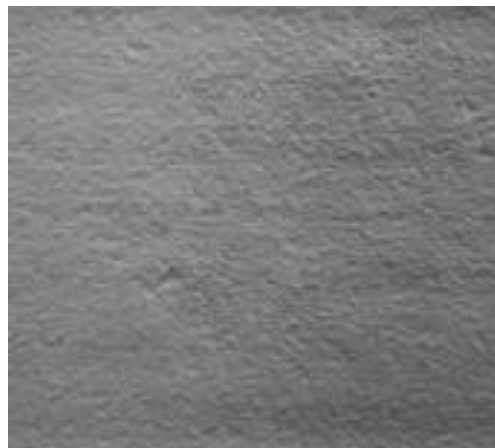
Figure 2.4 Example of CSP 3 (from ICRI 310.2R-2013)
