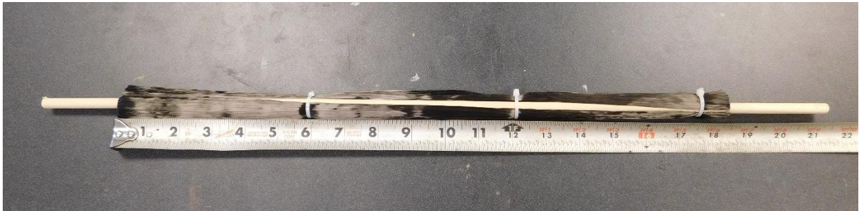
Figure 3.22 Assembled FRP Spike Anchor for Web Installation
