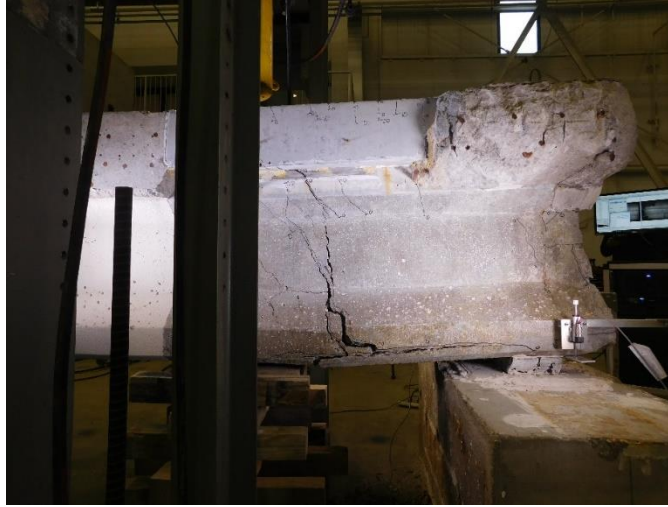
Figure 3.7 Damaged Specimen After Failure
