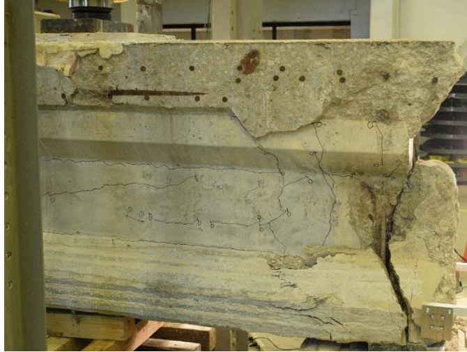
Figure 4.16 NSM Specimen After Failure
