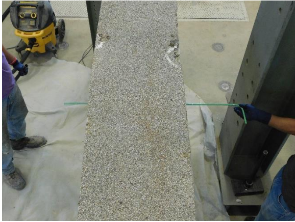
(e) No. 3 Bar Oriented for Bending Operation
