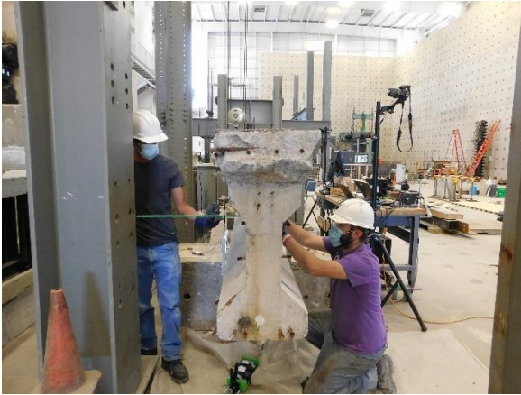
(c) Inserting No. 3 Bar Through Web
