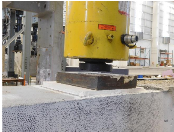
(c) Load Plate on Gypsum Concrete Wedge
