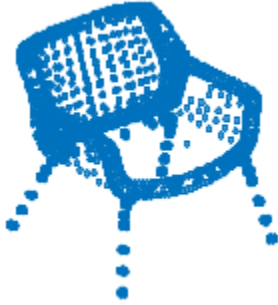
Figure 3.3. Example Set Data: a Point Cloud. This point cloud is a set of three dimensional coordinates \{(x_i, y_i, z_i)\}_{i=1}^n tracing out an object. We would encode this set by pre-specifying some ordering and arranging the coordinates as vectors in a matrix \mathbf{S} \in \mathbb{R}^{n \times 3} . The point cloud shown is from Meng, Yang, Ribeiro, et al. [27].
