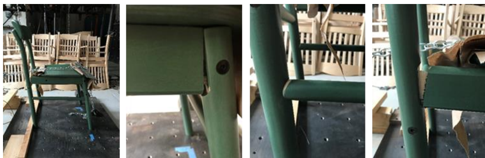
Figure 19. Chair C performance test failures
