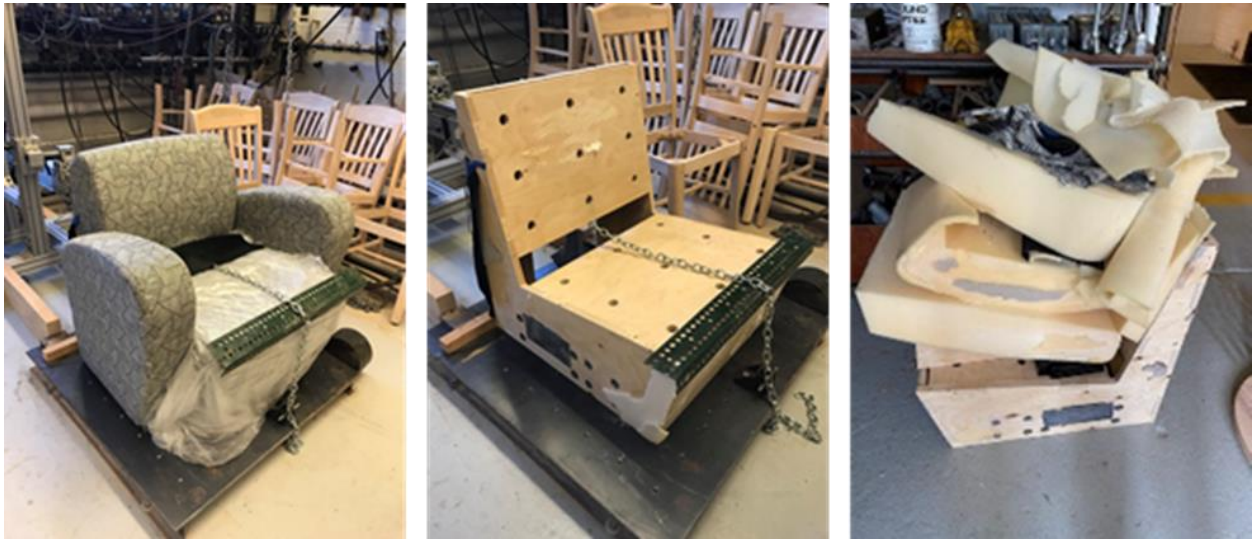
Figure 18. Chair B performance test failures
