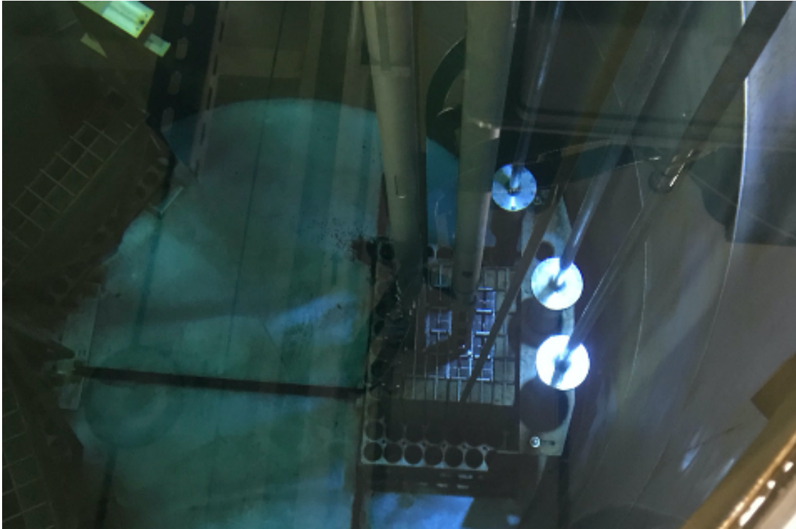
Figure 2.1. PUR-1 reactor, grid plate, coolant pool and detectors.
