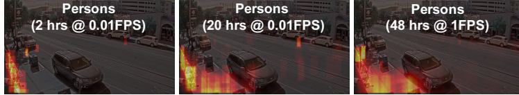
Figure 4.3. Class spatial distribution can be estimated from sparse frames sampled over long video footage. Among the three heatmaps: while sparse sampling over short footage (left) significantly differs from dense sampling of long footage (right), sparse sampling of long footage (middle) is almost equivalent to Video: Tucson (see Table 4.3).
