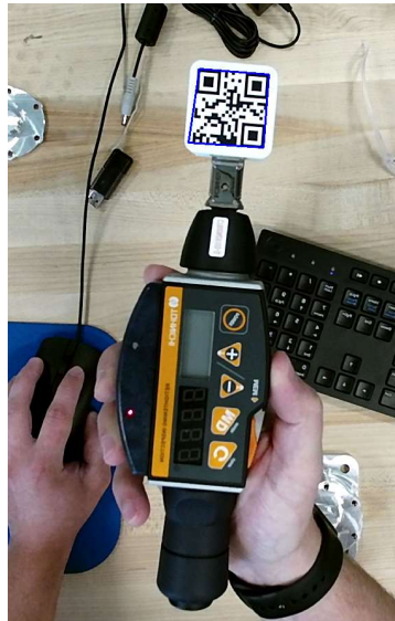
Figure 15. System detecting torque tool using QR code attached to the torque wrench.
