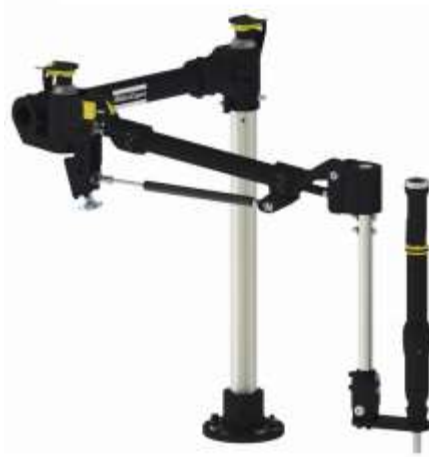
Figure 4. Atlas Copco Articulated Arm with Positioning Hardware (Atlas Copco, n.d.).
