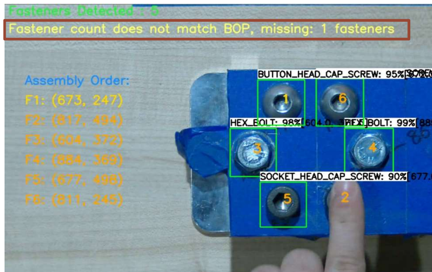
Figure 30. System Output Detecting Missing Fastener
