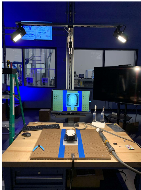
Figure 9. Assembly test setup with a camera hung over the assembly station.
