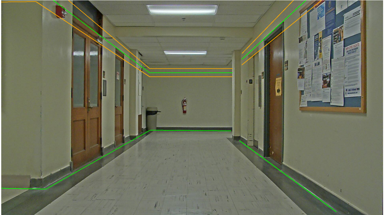
Figure 1.12. Projected walls with region boundaries. Green lines are the tops and bottom of walls projected at heights of 0 m and 2.2 m respectively, and the orange lines are the \pm 15 cm tolerances for the top.
