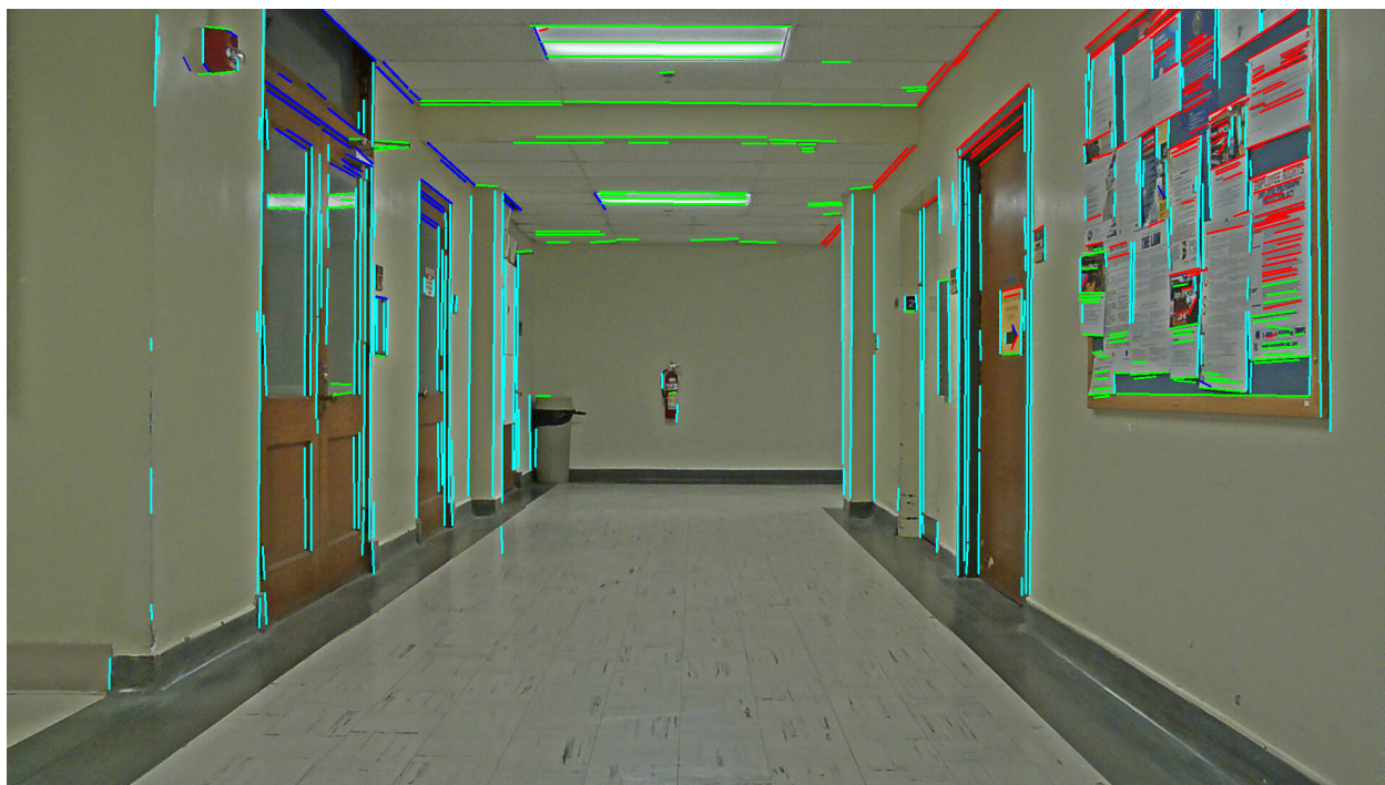
Figure 1.13. Line segment detections, color coded by their orientation. Green lines are horizontal. Vertical lines are teal. Blue lines have a downward slope. Red lines have an upward slope.
