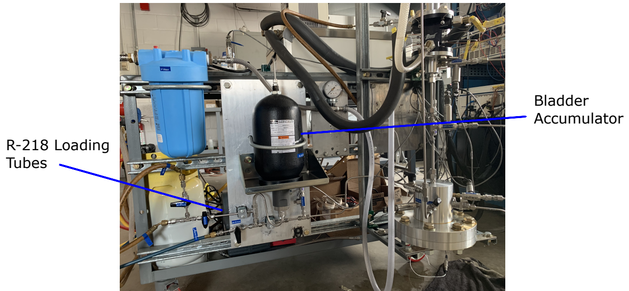
Figure 2.4. Nitrogen bladder accumulator.
