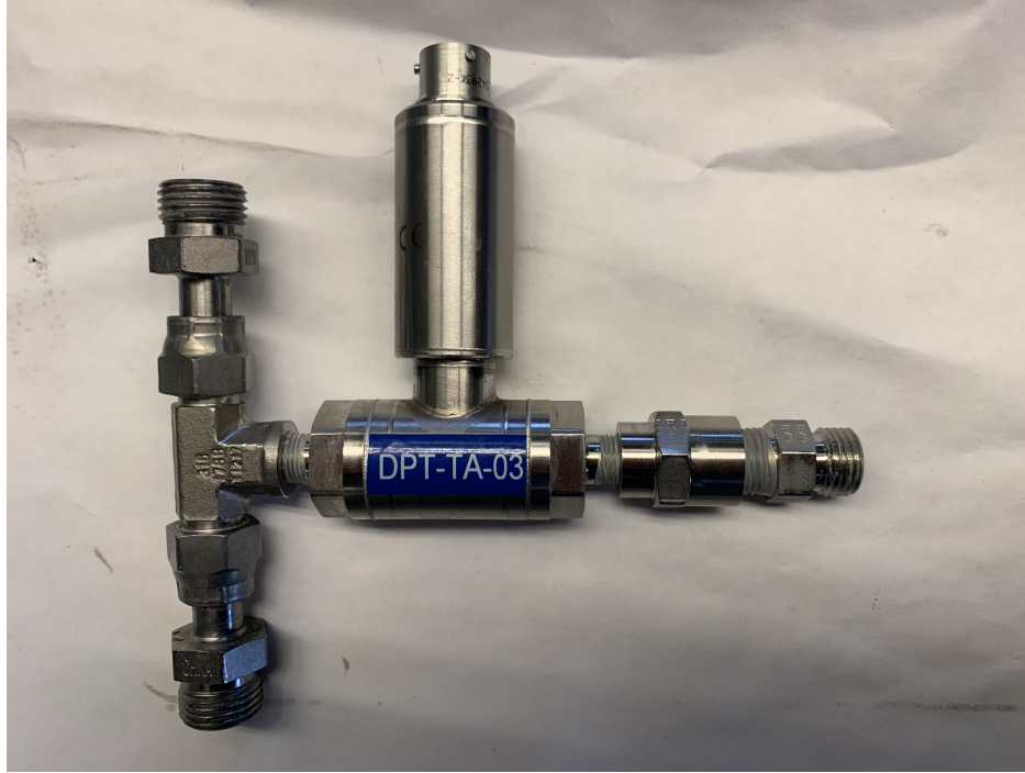
Figure 2.13. 6-4 LOHL6-S ZJ Installed in a DPT assembly.
