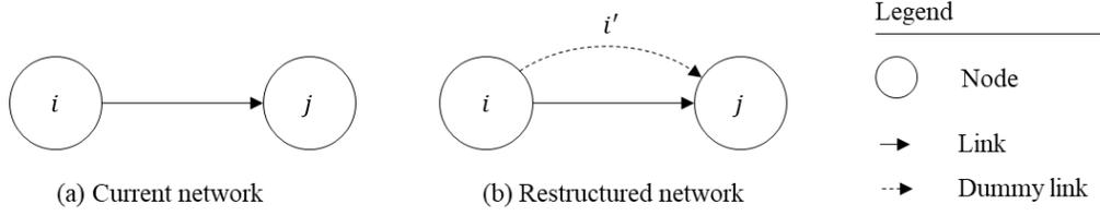
Figure 3-3. Transformation of the traffic network at links with AV-exclusive lane
