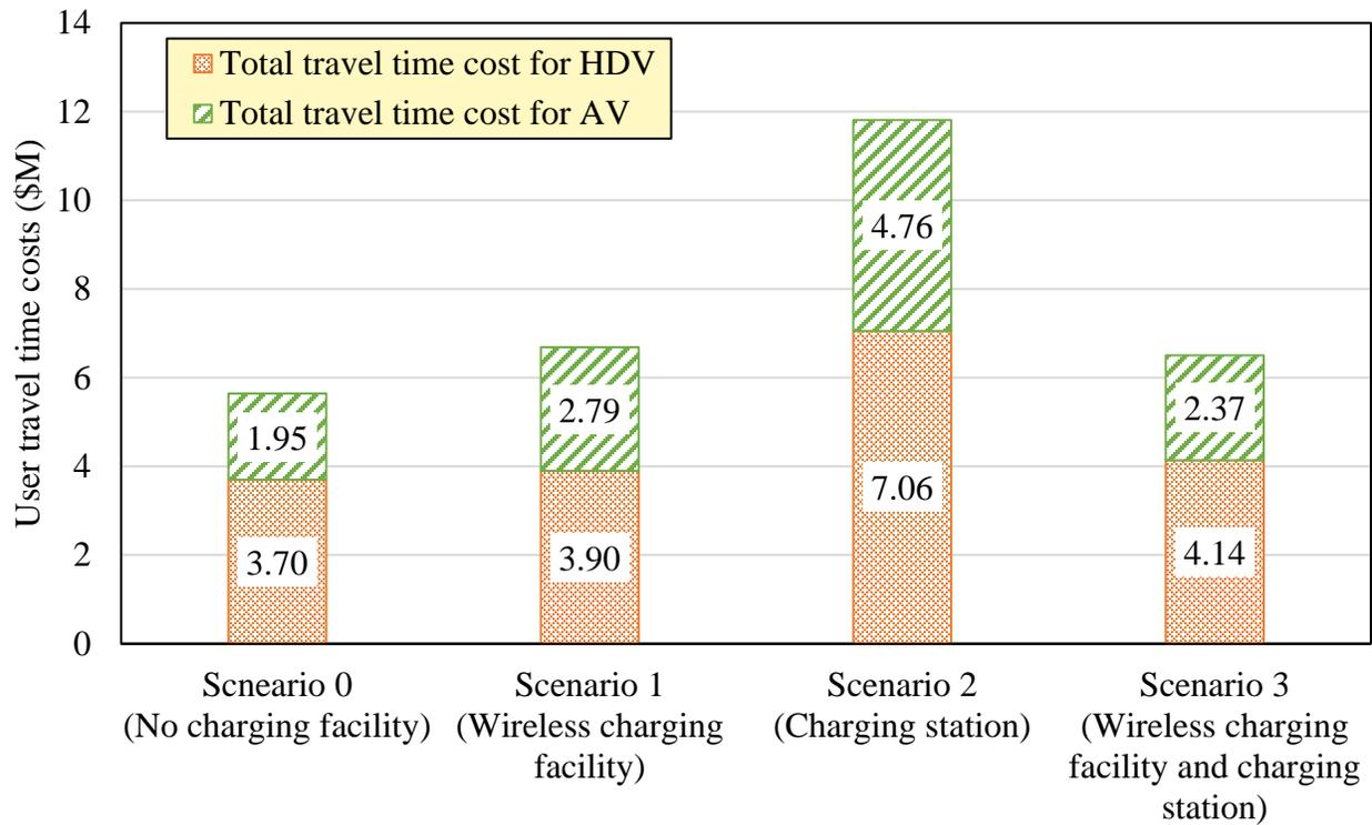
Figure 5-10. Comparison of the travel time cost of charging facility type scenarios
