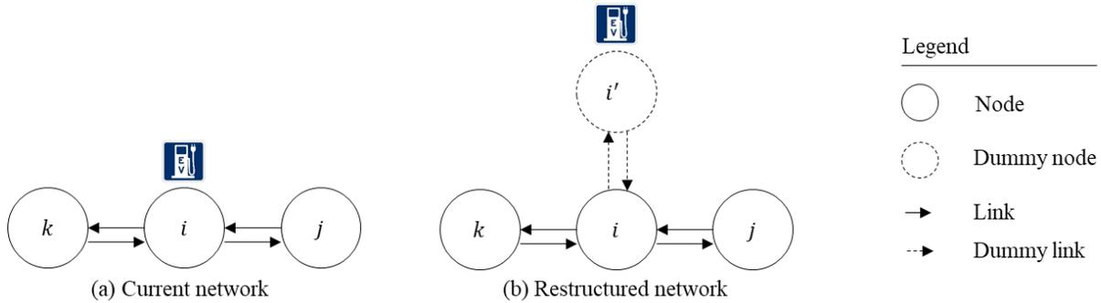
Figure 3-2. Transformation of the traffic network at nodes with charging stations
