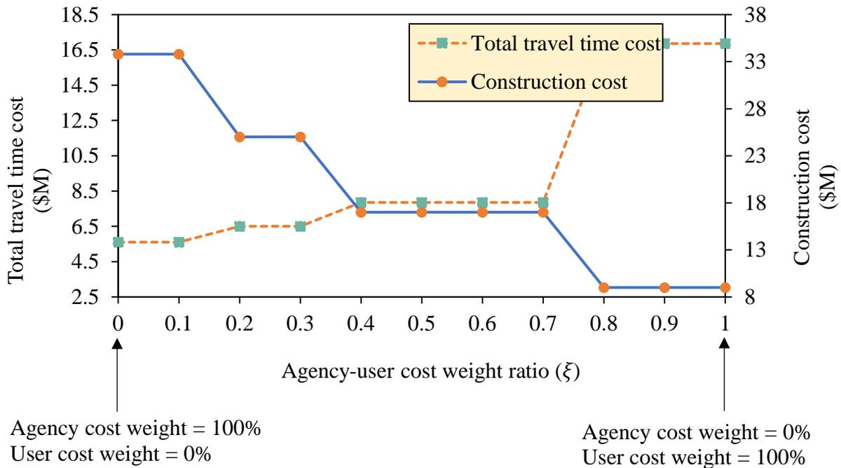
Figure 5-6. Impact of weights on the optimal costs
