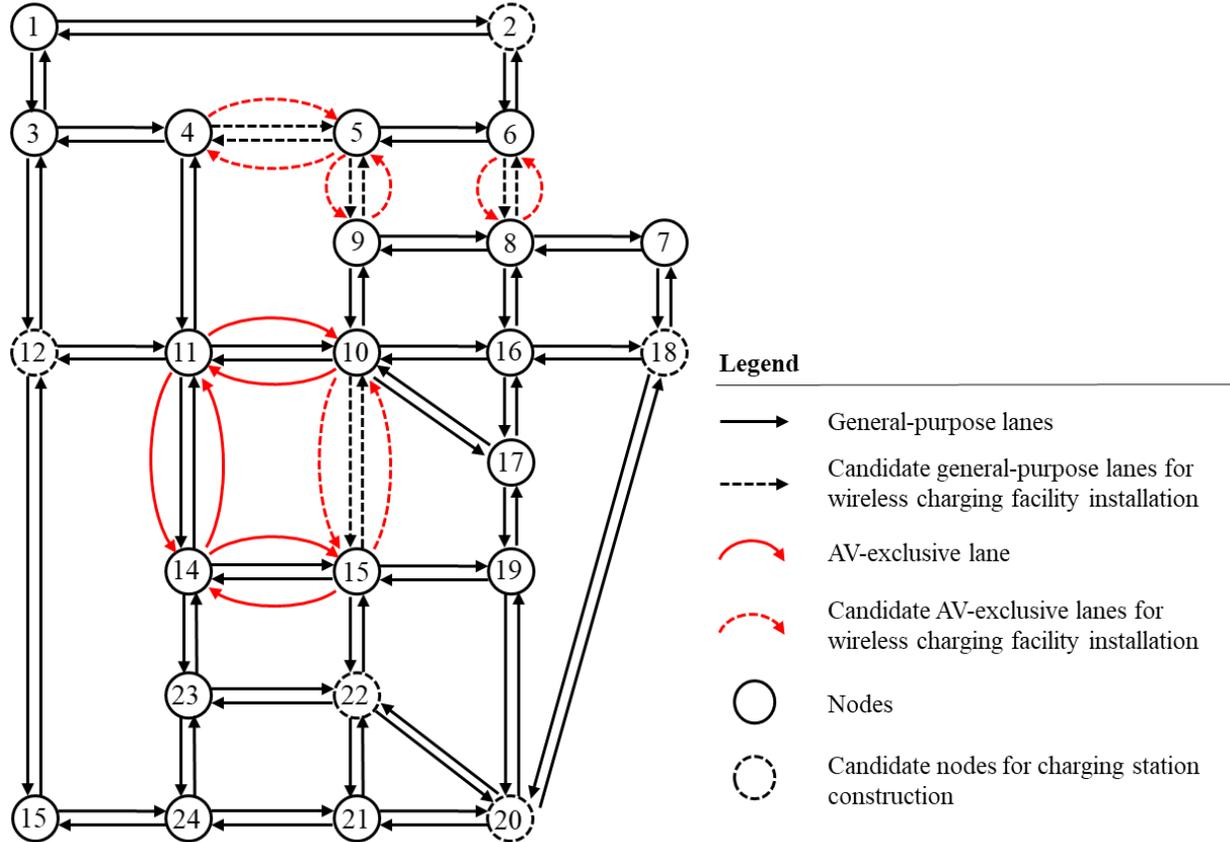
Figure 5-2. Candidate nodes and links for EV charging facility
