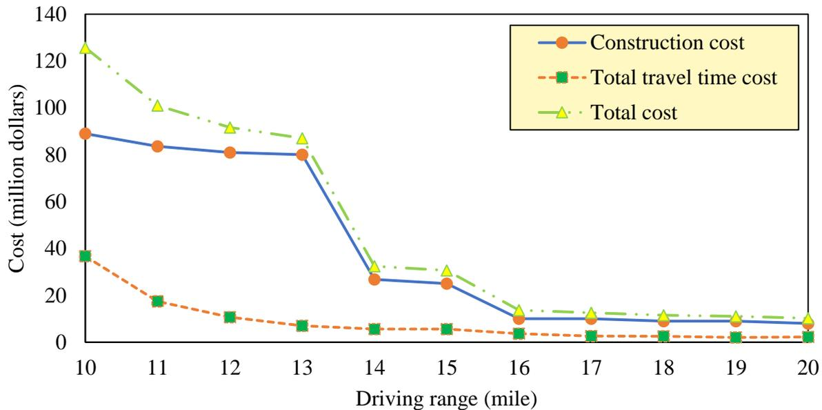
Figure 5-16. Impact of EV initial driving range on costs
