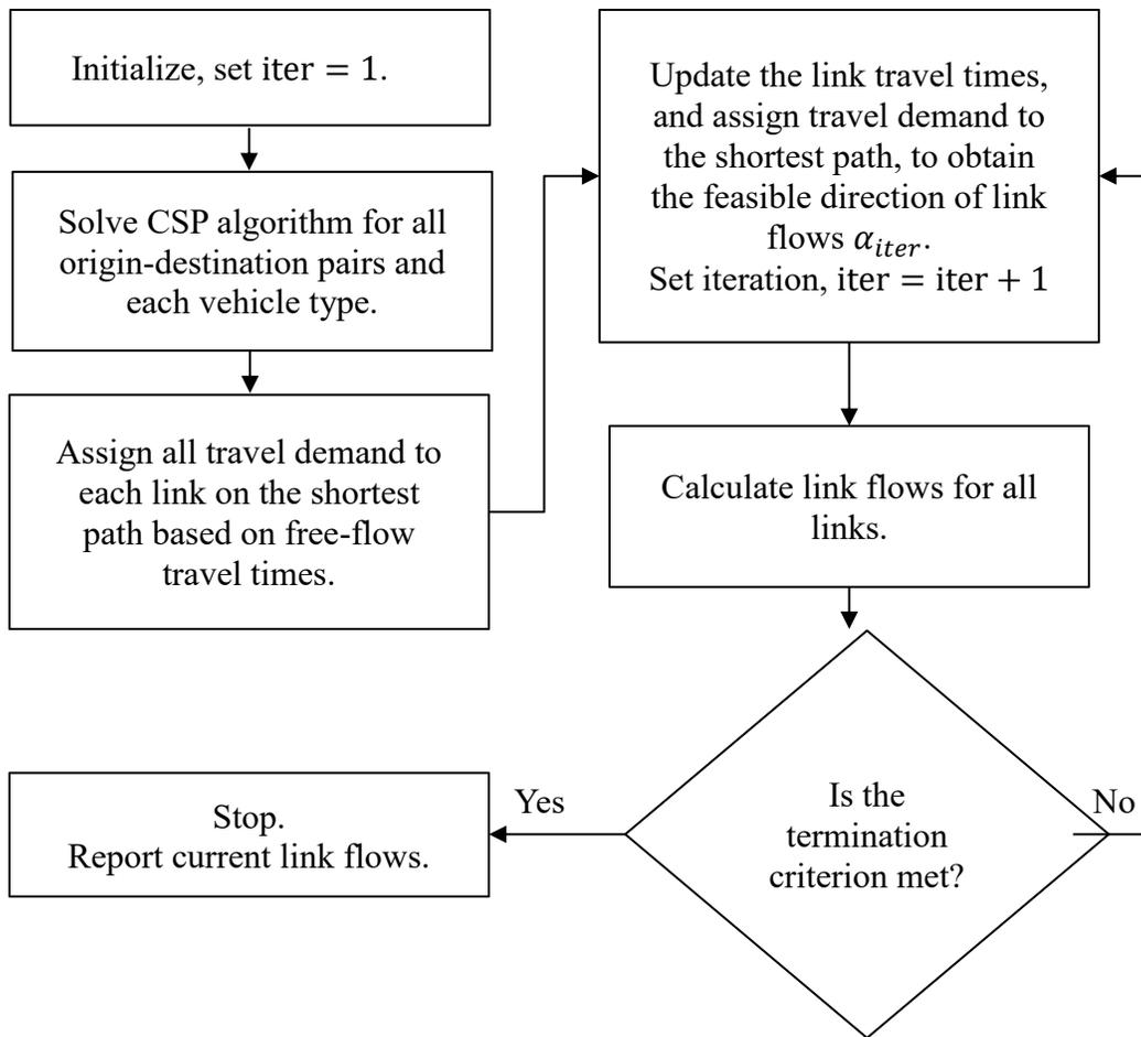
Figure 4-4. Lower-level solution flowchart
