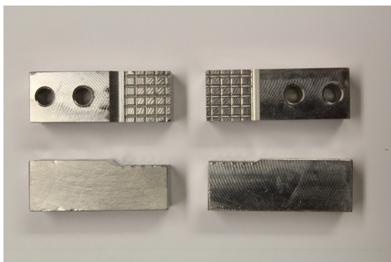
Figure 4.3. Two sizes of glue fixtures for use in the nano-precision tester.
