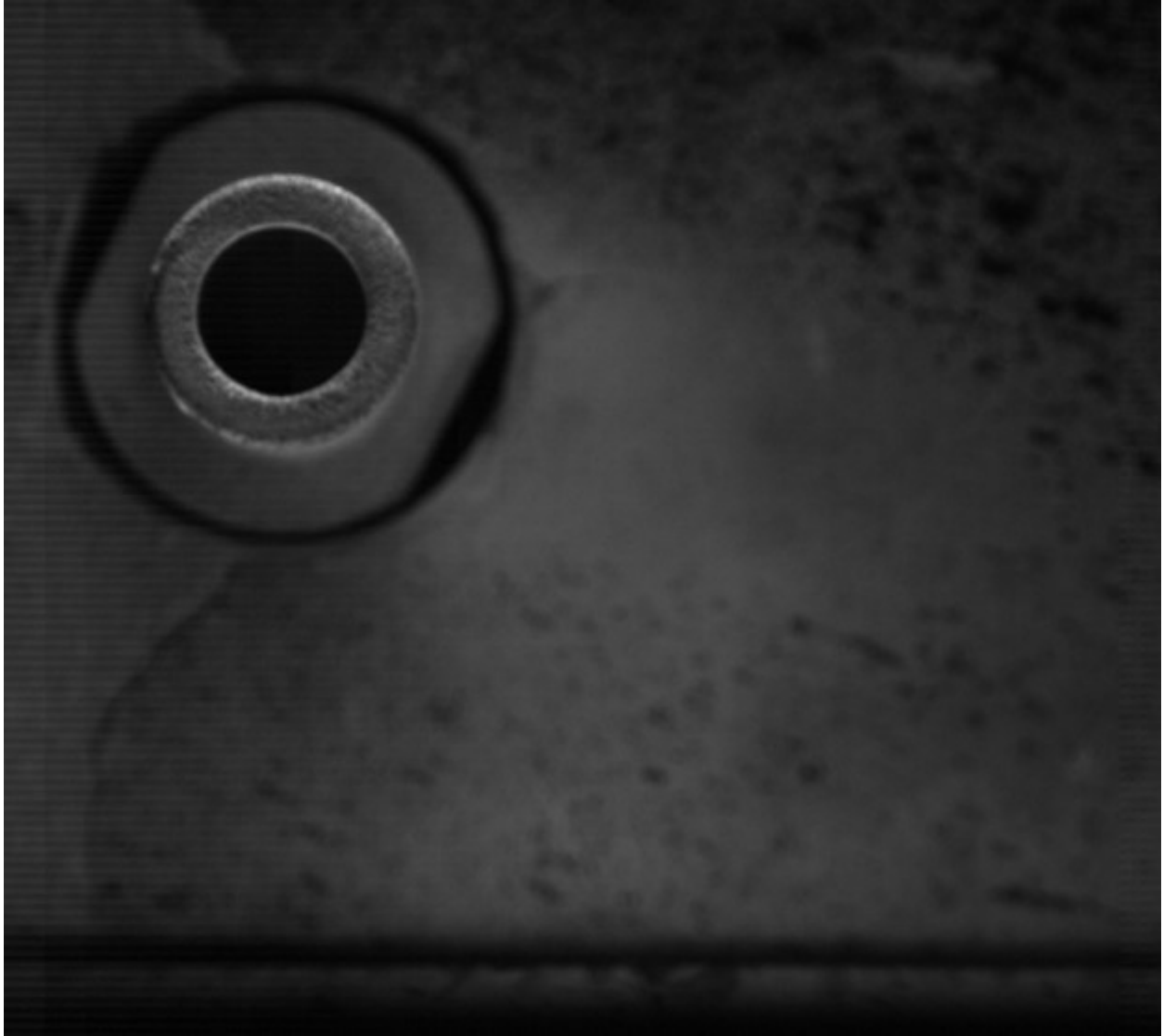
Figure 8.5. : Normal view of 5mm ID Injector, with the full image extents measuring 65mm across and 58mm down.
