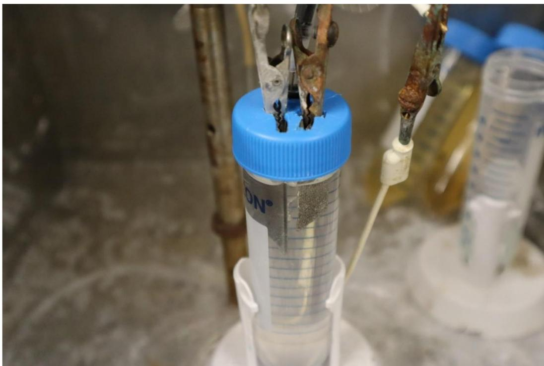
Figure 3.6. Image of 3 electrode electrochemical cyclic voltammetry test setup. The setup consisted of 1Ag/AgCl reference electrode, 1 platinum plate counter electrode, and the working electrode.
