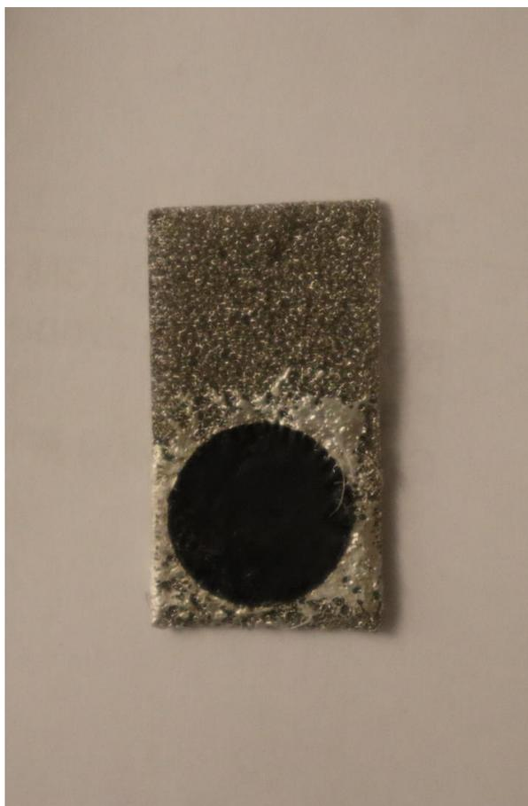
Figure 3.4. Image of completed electrode deposited onto nickel foam using conductive epoxy.
