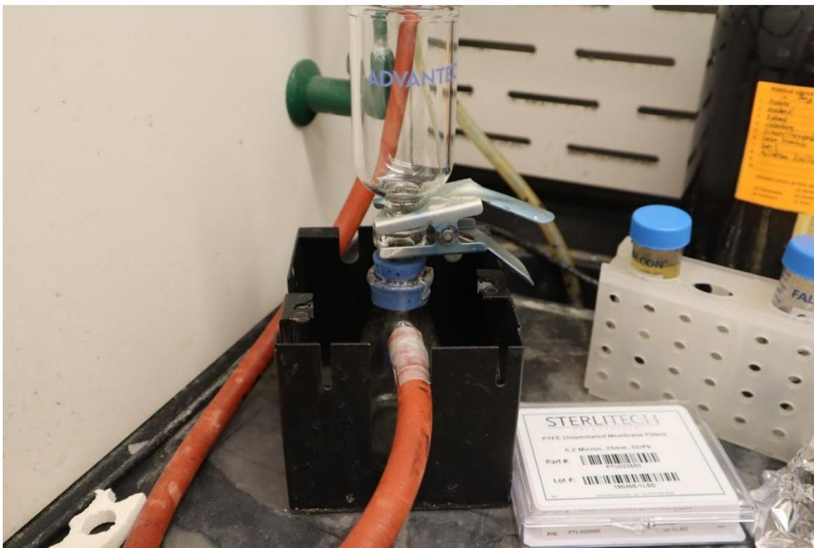
Figure 3.3 Vacuum Filtration process used to remove solute from sample to deposit electrode material onto membrane.
