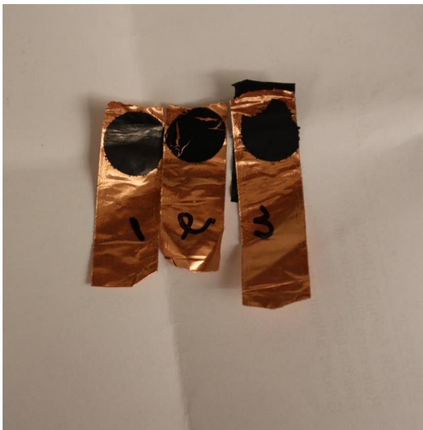
Figure 3.10. Samples deposited onto copper tape that showed large degrees of corrosion.
