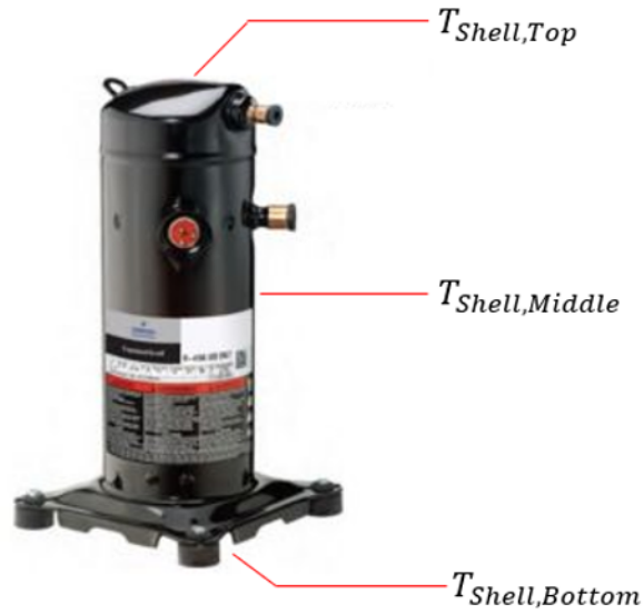
Figure 2.34. Compressor shell surface temperature instrumentation locations.
