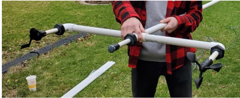
Figure 2.46. Close-up view of the weather station wind vane, anemometer, and light sensor.
