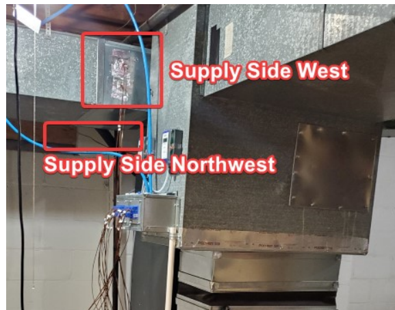
Figure 2.37. Thermocouple instrumented locations on the supply (west) side of the indoor unit.
