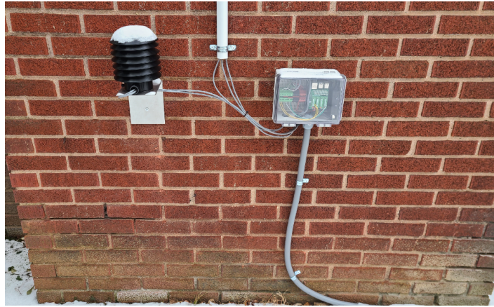
Figure 2.45. Waterproof Carflex conduit PoE routing from weather station controller to the DC House and connected radiation shield.
