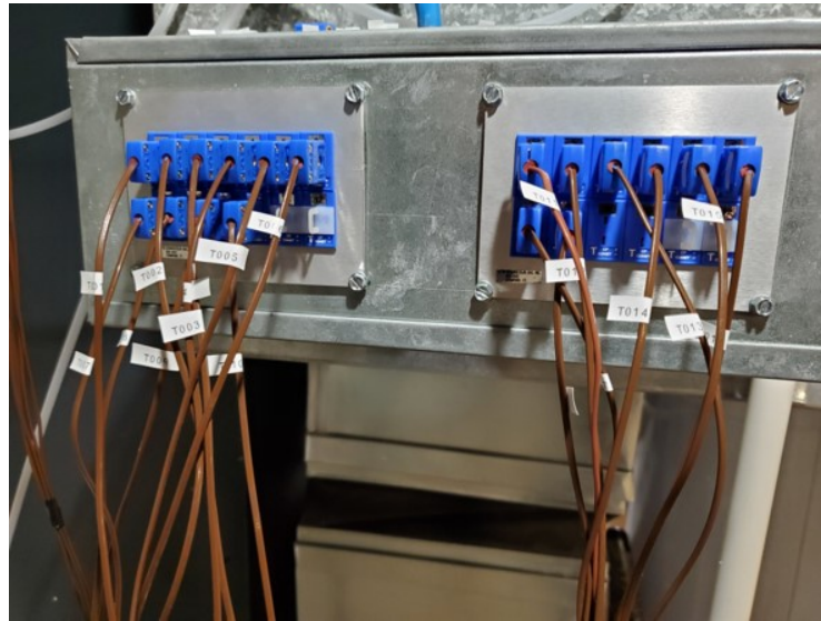
Figure 2.36. Yokogawa GM10 DAQ thermocouple interface panel.
