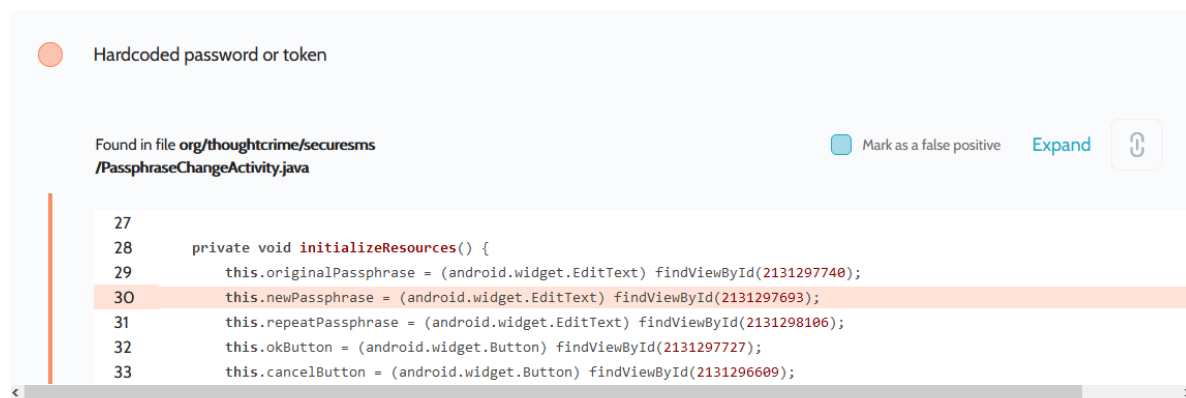
Figure 4.14. Detailed vulnerability report for a hard coded token vulnerability
