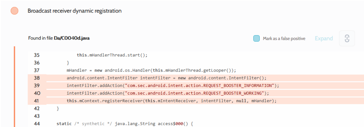
Figure 4.15. Detailed vulnerability report for a dynamic broadcast receiver registration
