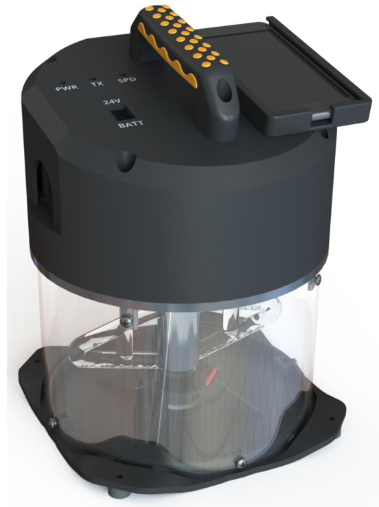
Figure 7.2. Rendering of a single detector system for portable spectroscopic and or dosimetric measurements.
