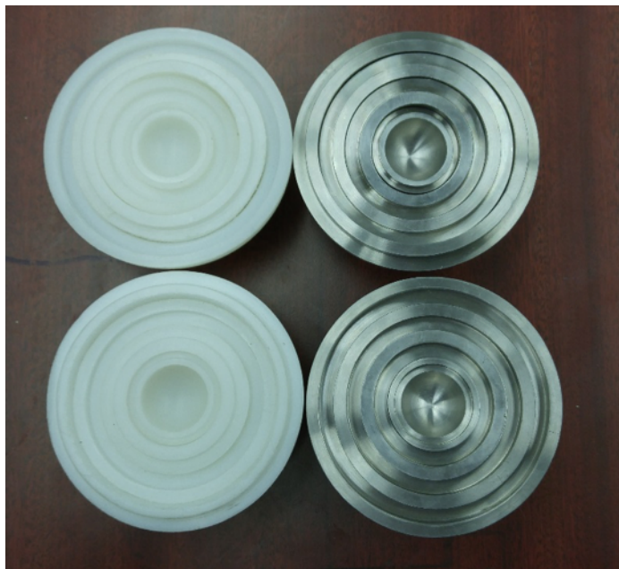
(a) Polyethylene and steel spherical moderating shells.
