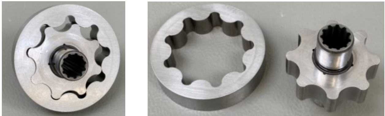
Figure 8.9. Photos of the first set of optimized gears in assembled and disassembled positions
