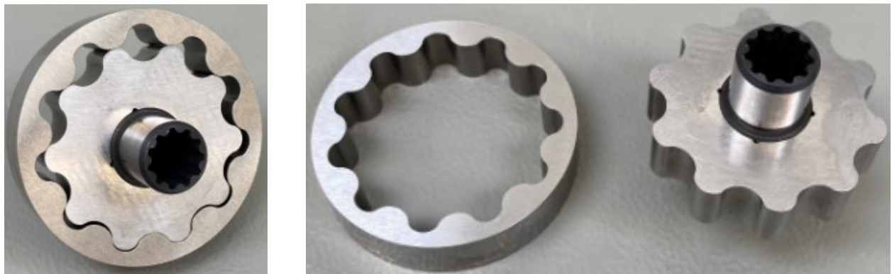
Figure 8.10. Photos of the second set of optimized gears in assembled and disassembled positions
