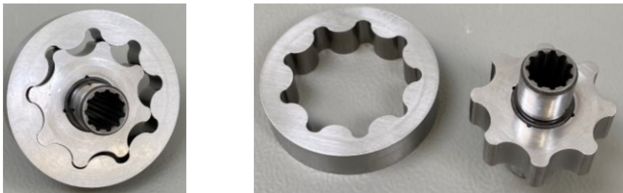
Figure 8.8. Photos of the reference gears in assembled and disassembled positions
