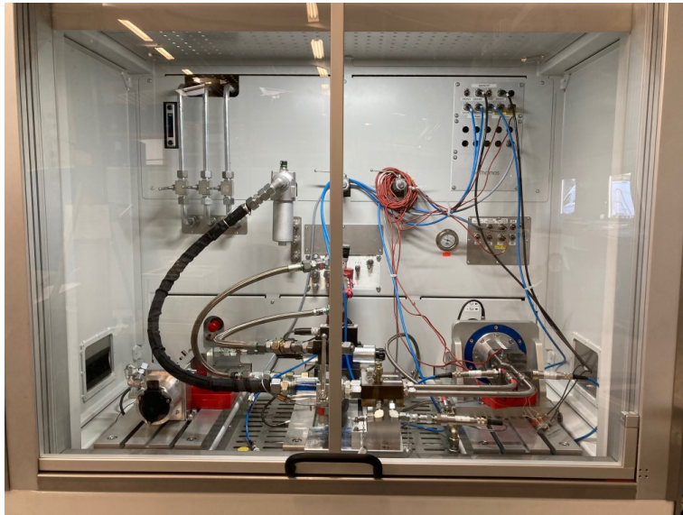
Figure 8.23. Photo of prototype pump mounted in the test stand
