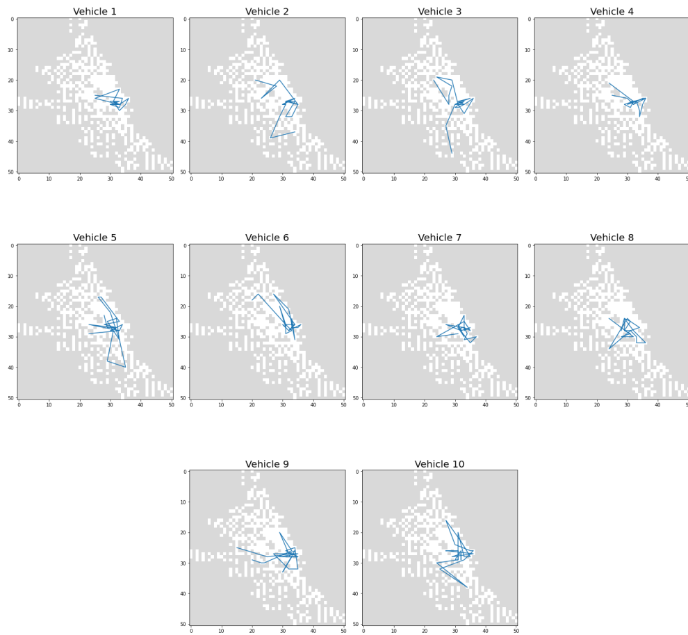
Figure 5.10. An example of routing trajectory of each vehicle under DeepBike strategy on Wednesday September 25, 2019
