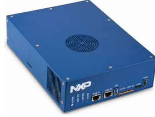
Figure 1. NXP BlueBox 2.0 ARM-based Automotive High Performance Compute (AHPC) embedded development platform. It delivers necessary prerequisites to help develop high-performance computing systems, analyze driving environments, assess risk factors, and then direct the car's behavior. BlueBox 2.0 also supports OpenCV applications using an external camera for real-time image classification object detection and image segmentation.
