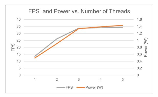
**Figure 4.5.** Relationship of FPGA Power Consumption to FPS as the Number of Threads is Increased During Deployment on FPGA
