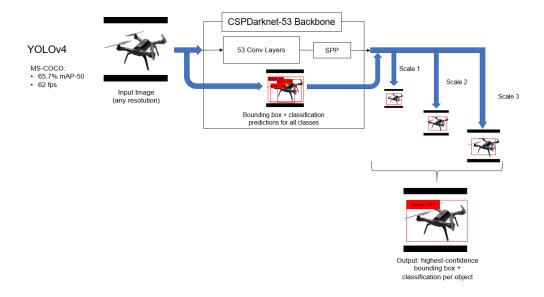
Figure 1.2. Model Architecture for YOLOv4 [28]. It consists of the CSPDarknet53 CNN backbone, an SPP module for fixed-length outputs, and the same head used in YOLOv3.
