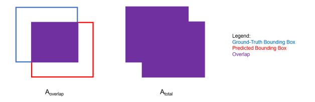
Figure 3.4. Illustration of IoU for Detection Accuracy
