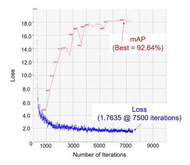
Figure 3.1. Model mAP-50 and Loss versus Number of Training Iterations
