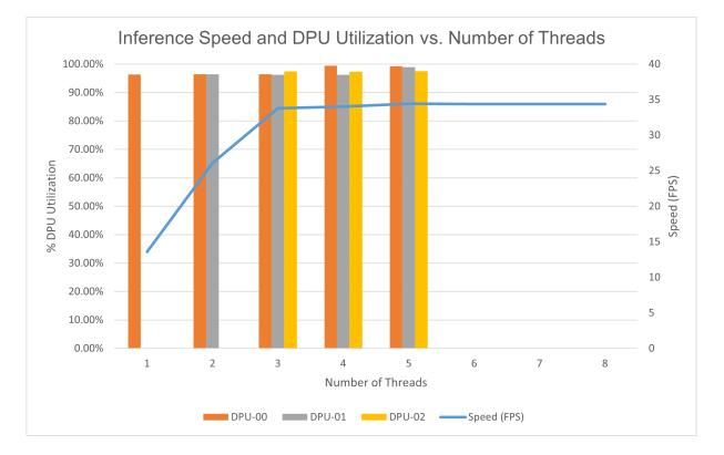
Figure 4.3. Comparison of Speed in FPS and DPU % Utilization to Number of DPU Threads varied from 1 to 8
