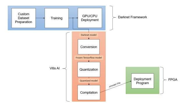
Figure 3.2. Experimental Workflow
