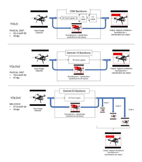
Figure 1.1. Model Architecture for YOLO [9], YOLOv2 [21], and YOLOv3 [22]. Each model is a single-shot object detector, but underlying changes to the CNN backbone allow for improvements in speed and accuracy with each iteration.
