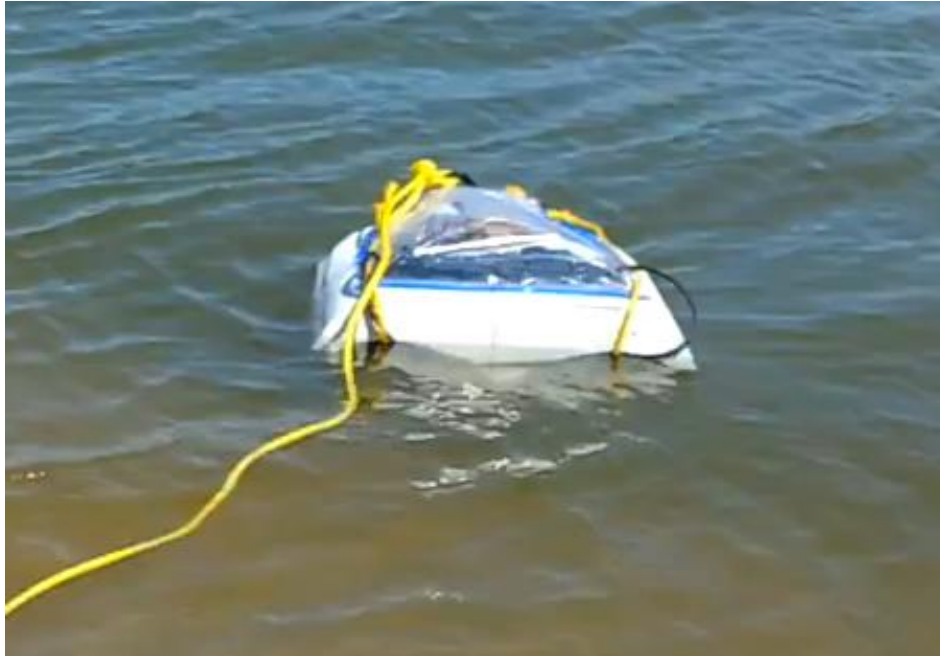
Figure 2.12. Final prototype floating in Lake Harner. The USV floats at the desired level, such that the thrusters are completely submerged in the water. The retrieval tether seen is a 0.5-inch polypropylene rope, used to pull the USV to shore in case of failure during testing.
