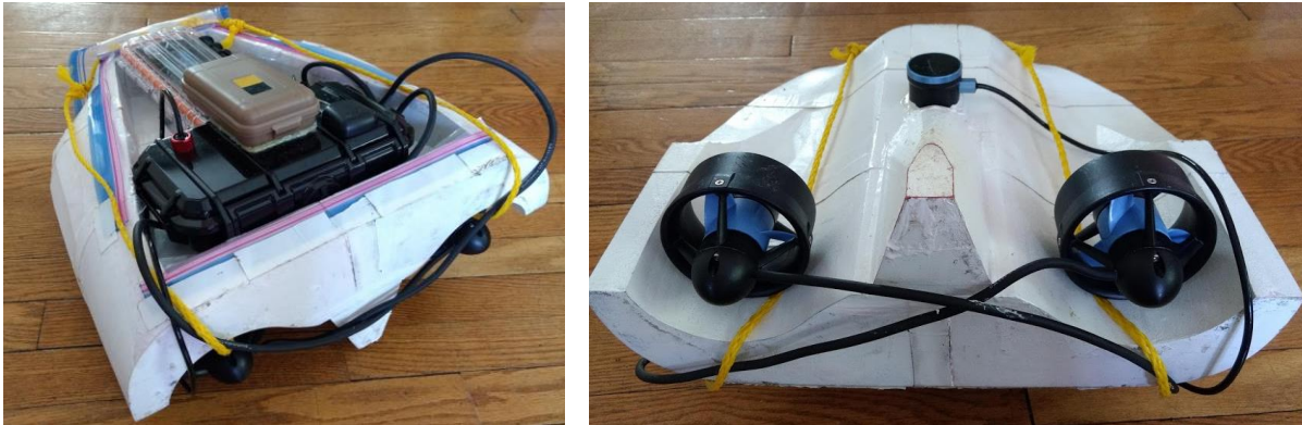
Figure 2.8. Picture of final working prototype. The final USV weighs 14.2 lbs with all including components. The thrusters and sonar sensor were placed below the USV structure, while the battery and all other electronics were placed in waterproof containers on top. A waterproof antenna for the GPS was placed outside the container for a better signal.
