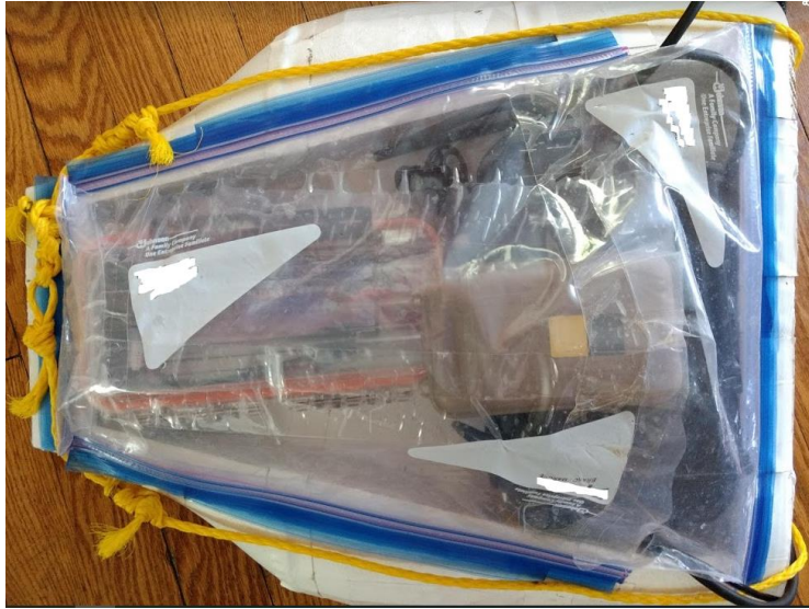
Figure 2.11. Water splash shield and rope frame. The splash shield was made from re-sealable plastic bags, providing a press fit cover and easy access to the electronics container. While the splash shield is not waterproof, it significantly reduced the amount of water entering the upper cavity. The rope frame was tightened around the boat and acted as an attachment point for the retrieval tether.
