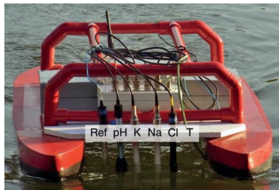
Figure 1.5. Remote controlled catamaran floating in Cegielnia pond in Gliwice, Poland. Select probes attached to the back analyzed water quality [13].
