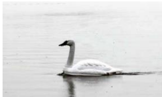
Figure 1.3. NUSwan driving in a local reservoir in Singapore. The prototype utilized only GPS to navigate [10].
