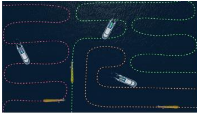
Figure 1.9. Sample scenario of three USVs acting as recharge stations for AUVs. Simulations and field experiments are performed to test algorithms [17].
