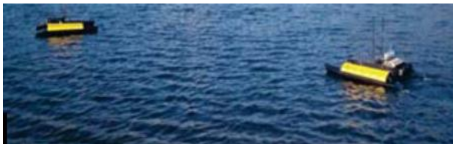
Figure 1.8. Two ASVs deployed in a local reservoir in Durango, Colorado. One is equipped with water quality sensors and the other with a water sampling apparatus [16].
