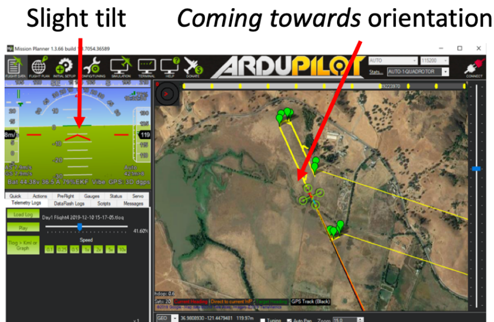
Figure 2.14. UAS controlled by Mission Planner software, showing UAS attitude is slightly tilted, leading to performance decrease while the UAS is coming towards the GCS.
