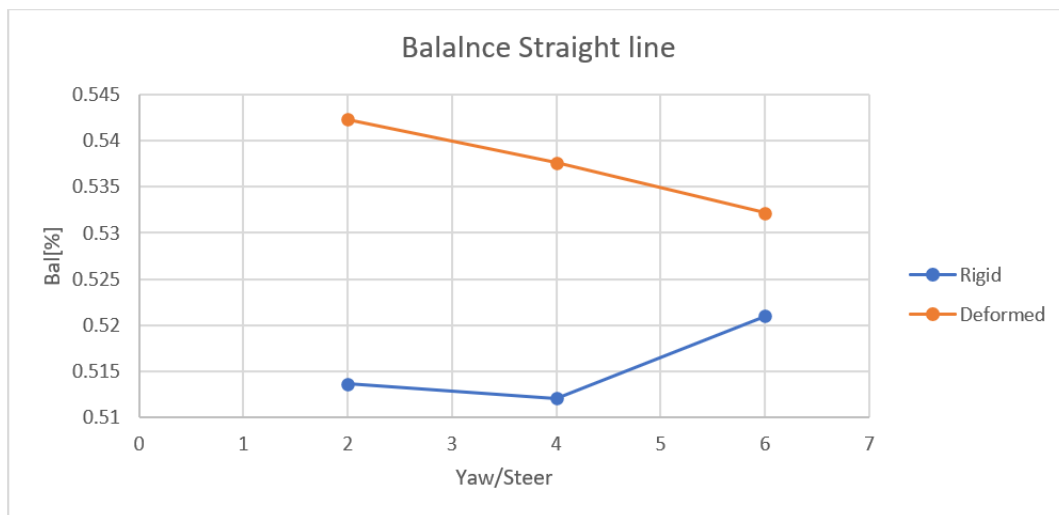
Figure 4.11. Rigid VS Deformed yawed flow domain Balance
