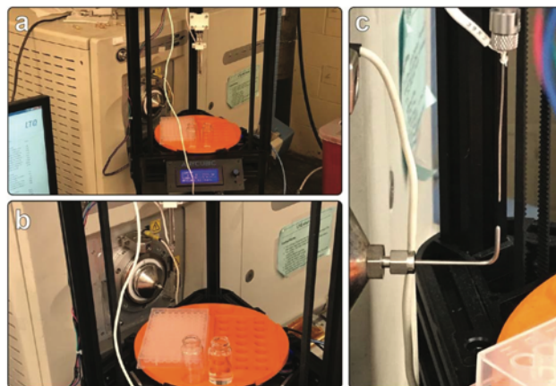
Fig. 1 Photographs of (a) the device in its home position in front of the mass spectrometer, (b) the custom syringe assembly moved to the spray position, and (c) a closeup of the syringe in the spray position showing the 90° bent capillary.
