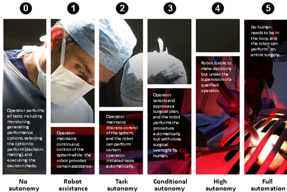
Figure 2.2. Classification system for autonomous systems in surgical robotics. Image taken from [46]
