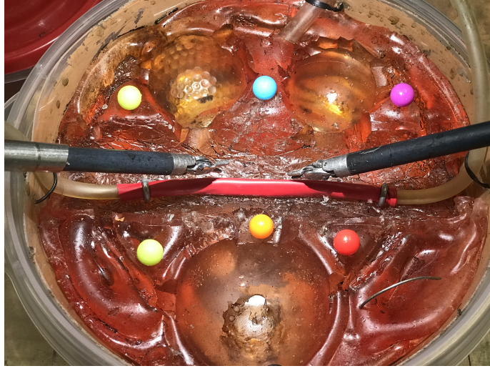
Figure 3.7. Calibration markers used to calculate homography transformation.
