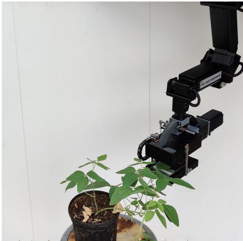
Figure 4.1 The 6 DOF robotic arm with LeafSpec attached during leaf scanning.
