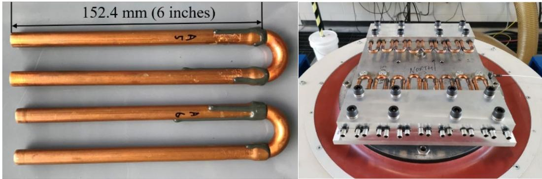
Figure 4.11. Photographs of the U-shape joints with adhesive (left) and the fixtures containing a set of 8 samples each installed on the vibration shaker test stand.
