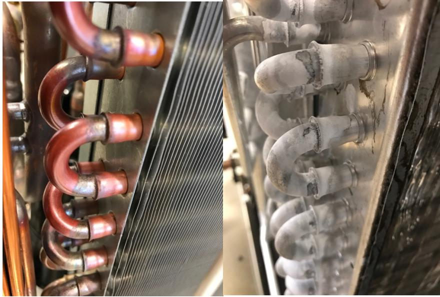
Figure 4.3. Copper and aluminum U-joints used in the tube-and-fin heat exchangers
