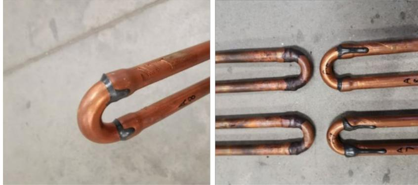
Figure 4.13. Photographs of the U-shape joints after the vibration test for adhesive joints(left) and vibration joints compared with brazed joints (right).
