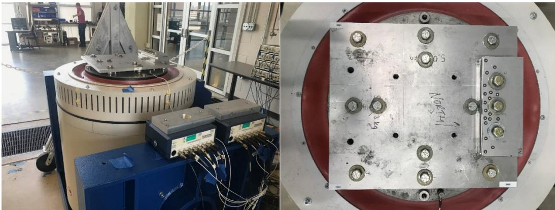
Figure 4.9 Pictures of the shaker test stand (left) and its base plate (right)
