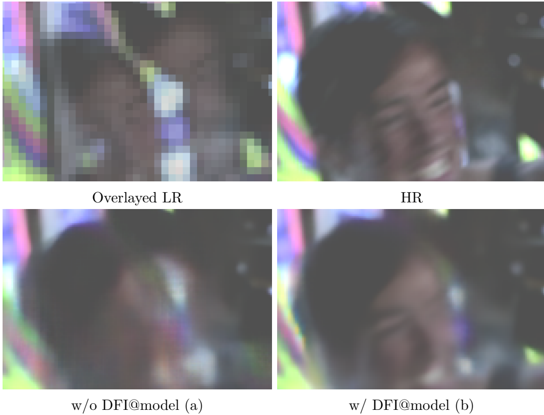
Figure 6.12. Ablation study on feature interpolation. The naive feature interpolation model without deformable sampling will obtain overly smooth results for videos with fast motions. With the proposed deformable feature interpolation (DFI), our model can well exploit local contexts in adjacent frames, thus is more effective in handling large motions.
