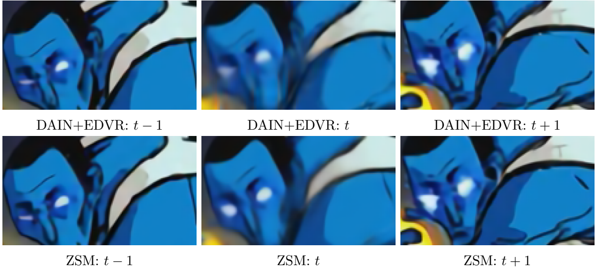
Figure 6.15. Temporal inconsistency issue in STVSR. It is more difficult to synthesis HR frame t than HR frames: t - 1 and t + 1 , since LR frames: t - 1 and t + 1 are available and LR frame t is missing during testing. Synthesized HR frame at the time step t is more blurry with fewer visual details than results at t - 1 and t + 1 .
