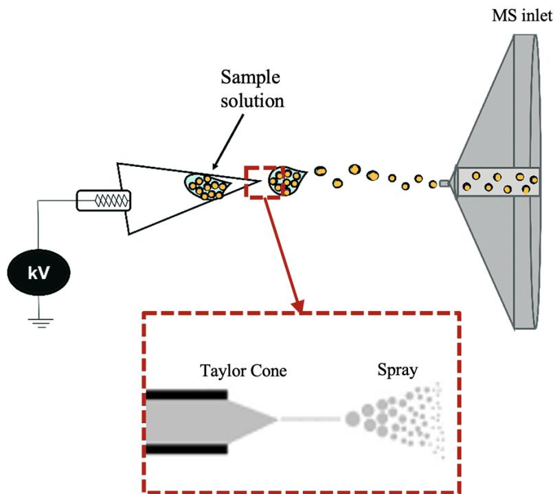
Figure 2.1 Paper spray mass spectrometry spray mechanism. Solvent and voltage applied to the dried sample on paper substrate in front of MS inlet, resulting in ionization occurs under ambient conditions.
