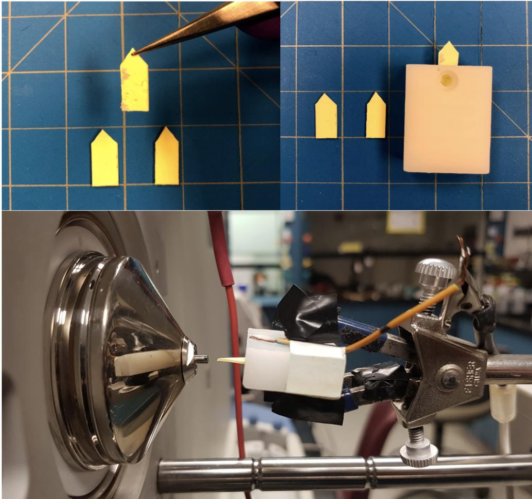
Figure 2.1 A) Paper spray tip preparation with sample collected on concrete surface, B) paper tip inserted into milled Delrin cartridge and C) placed 3-4 mm from the inlet.
