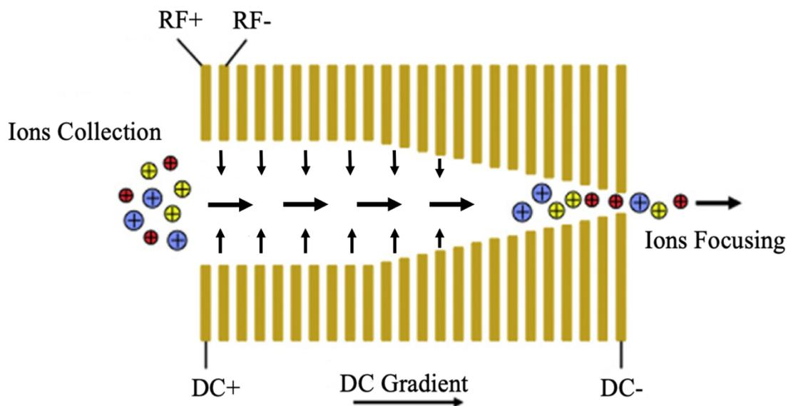
Figure 3.2 Schematic of the ion funnel with RF potentials of equal magnitude and opposite phase applied to alternate electrodes and DC potentials applied to each electrode.
