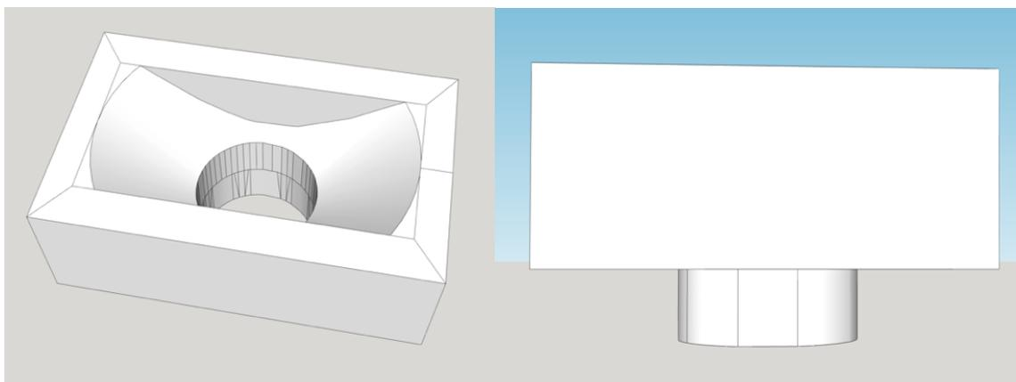
Figure 5.2 3D design of new snap-in SPE column to hold more SPE materials.
