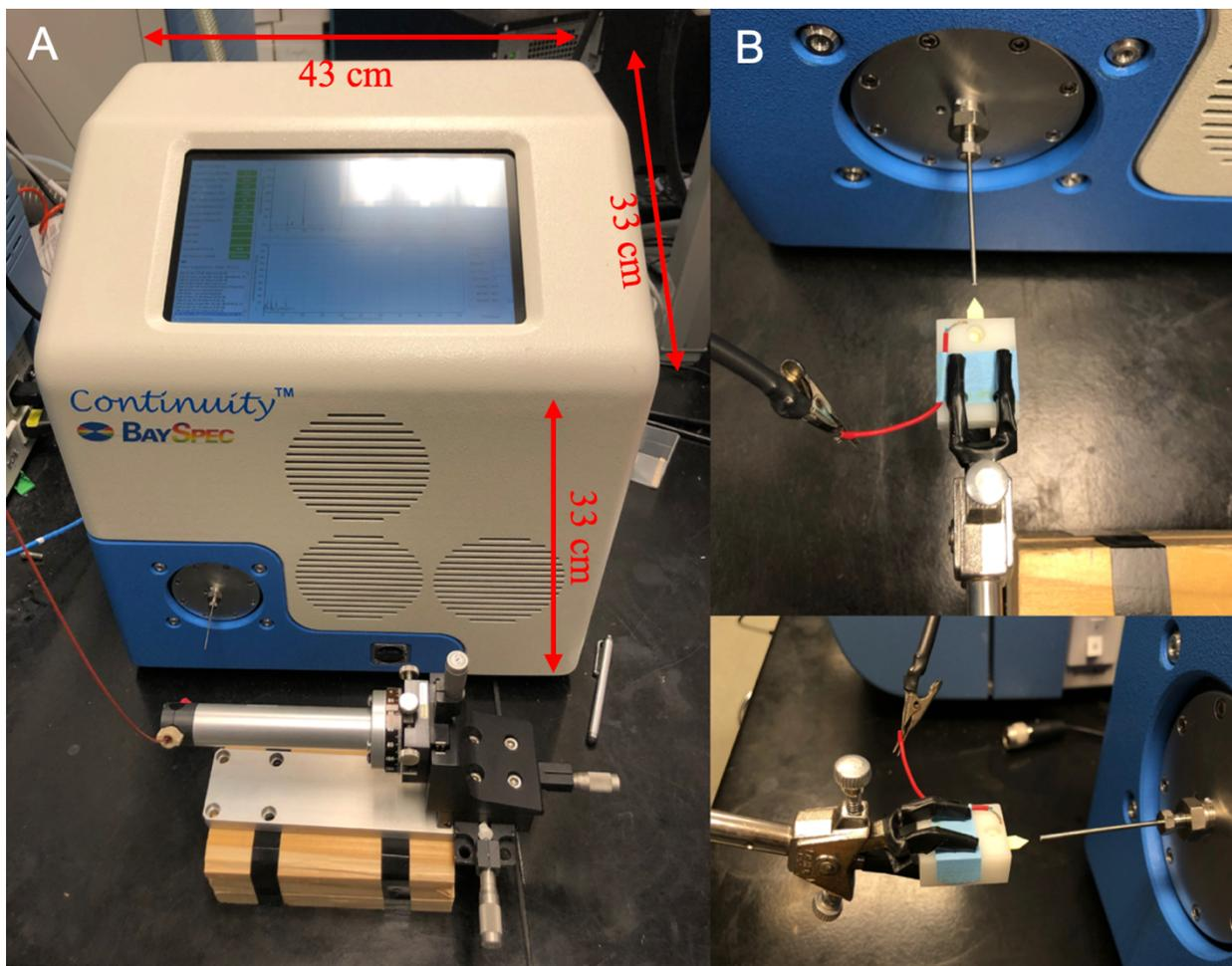
Figure 3.1 A) BaySpec Continuity Mass Spectrometer with electro spray ionization set-up for calibration and optimization and B) PS set-up with PSA paper ticket inserted into Delrin cartridge and positioned 1 mm from the MS inlet.
