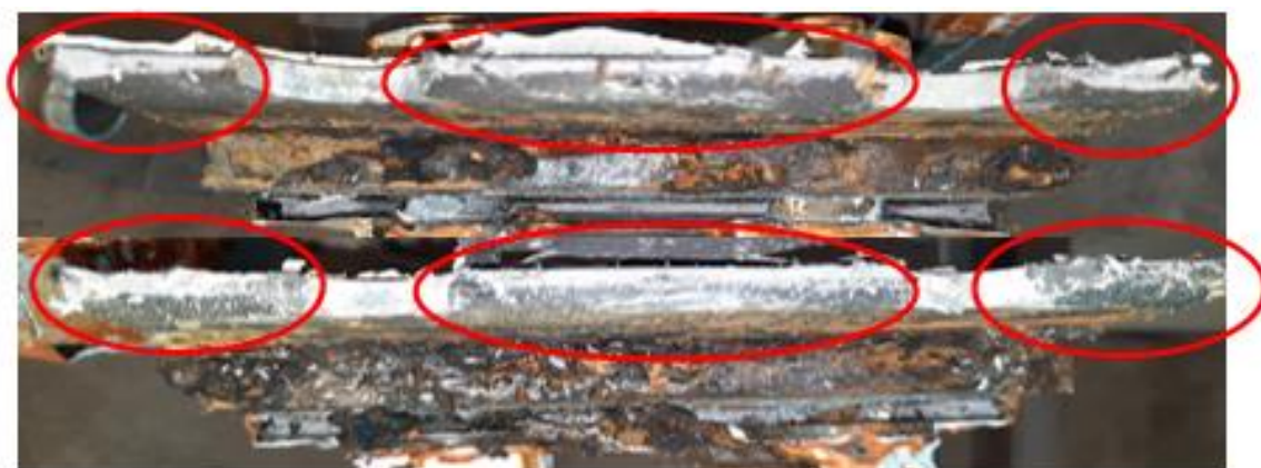
Figure 5.6. Specimen 19 cross-sectional area, exposed to 284 days of corrosion.
