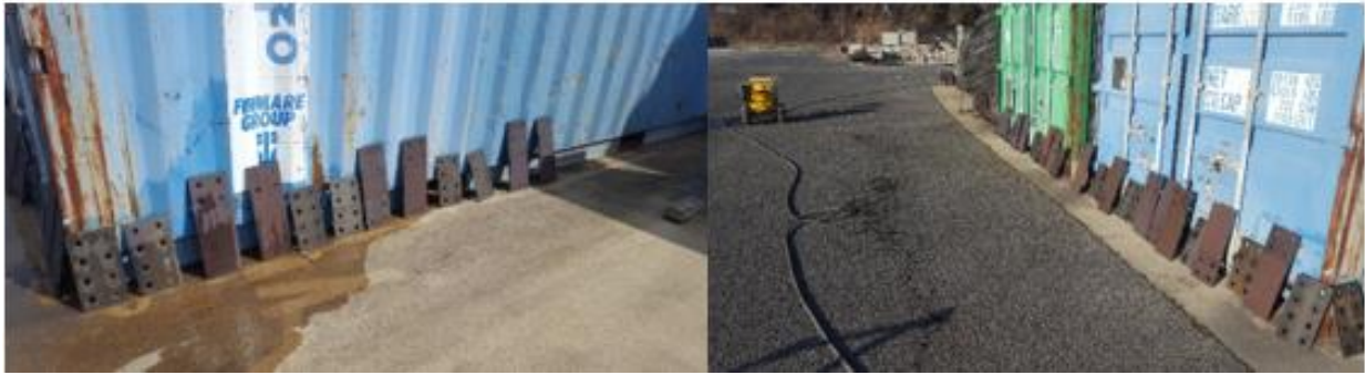
Figure 4.10. Plate's dirt removal with a 3800-psi pressure washer.
