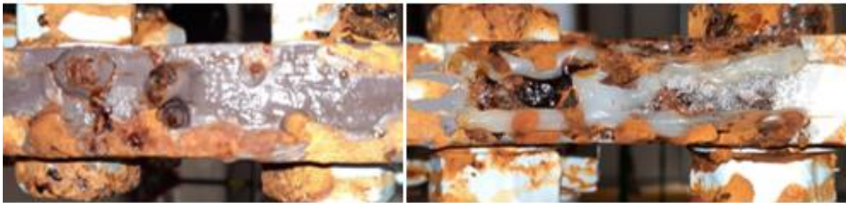
Figure 5.3. Black rust in Termarust (left) and caulked (right) specimens for Condition B.
