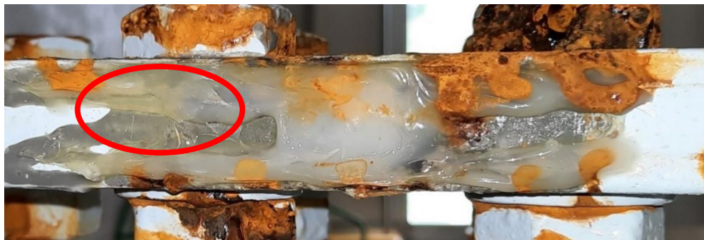
Figure 5.2. Discoloration of caulked specimen.
