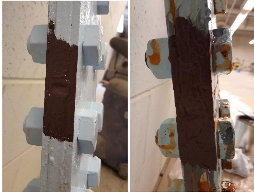
Figure 4.21. Termarust application for initial and repair condition.
