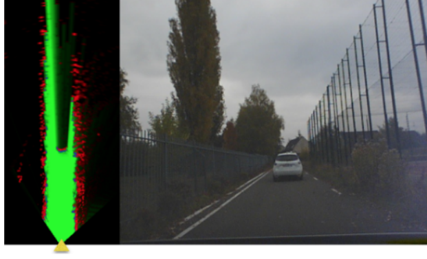
Figure 4.5. A scene with corresponding evidential occupancy grid [33].
