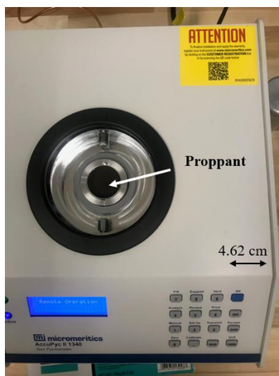
Figure H.3. (a) pycnometer used to measure proppant density; (b) density measured
