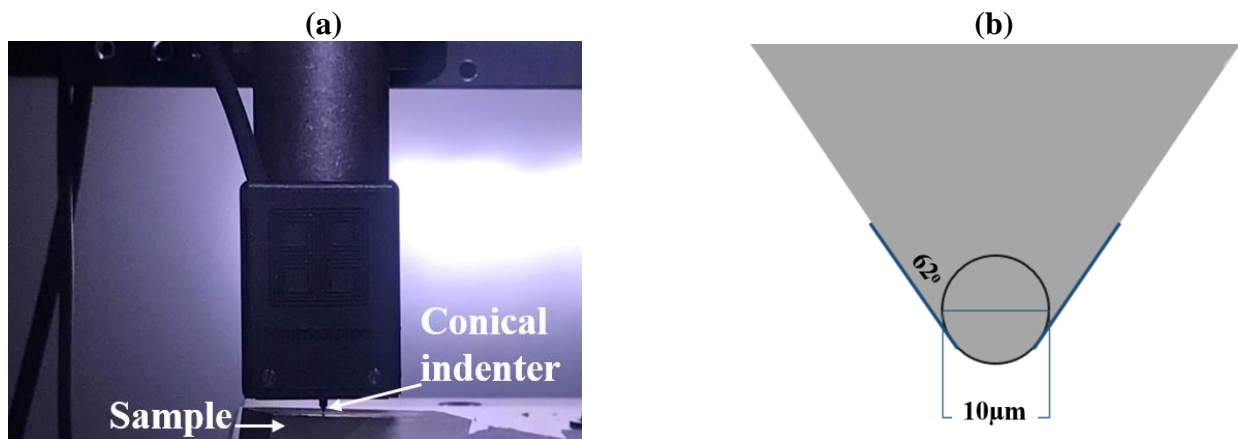
Figure 5.10. (a) Micro-indenter & sample setup; (b) schematic of the micro-indenter employed
