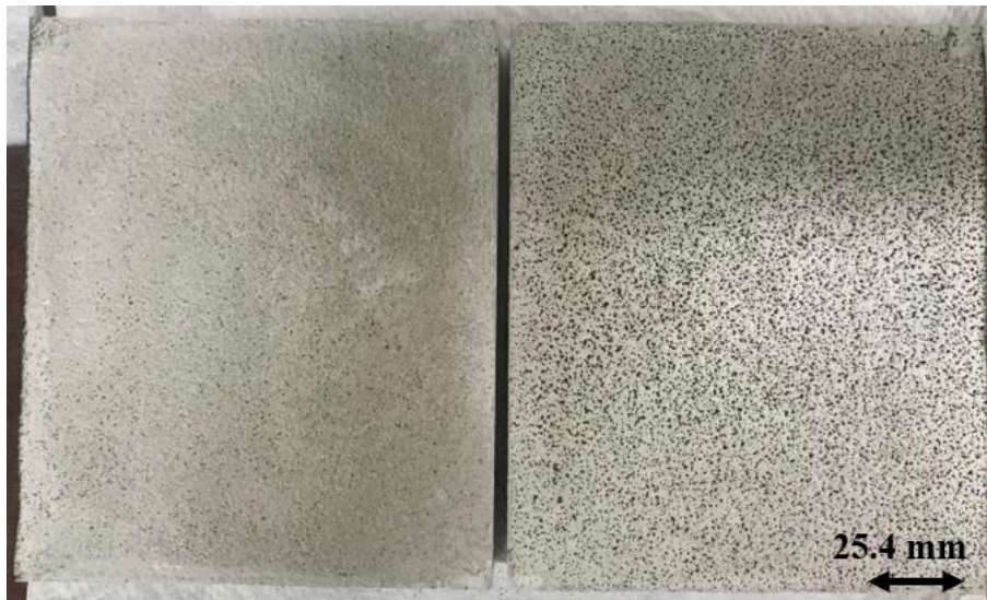
Figure H.8. Sample embedded with proppant in the discontinuity GE w
