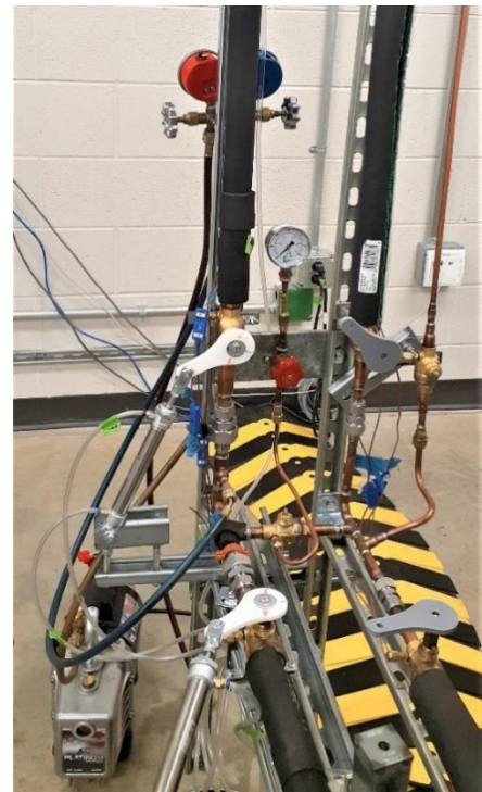
Figure 3.18: Evacuating the test sections before charging back with refrigerant
