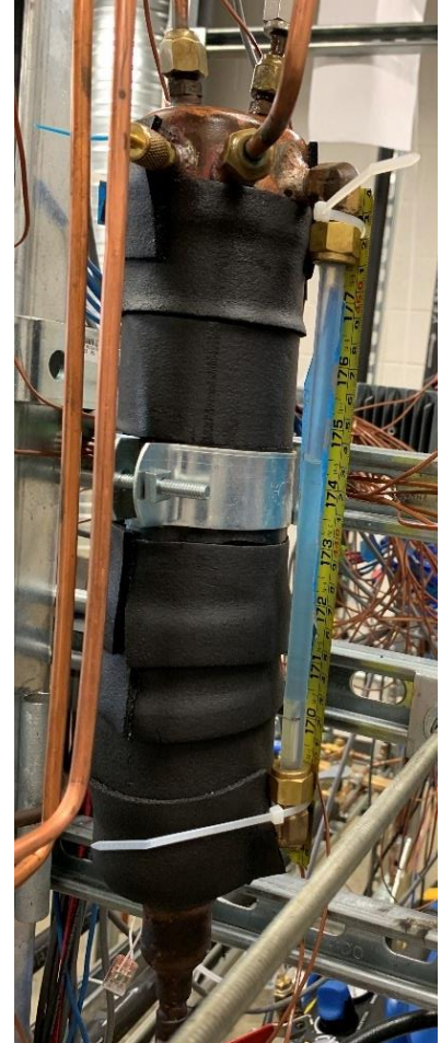
Figure 3.14: Picture of sight tube connected in parallel to the oil collector for monitoring level
