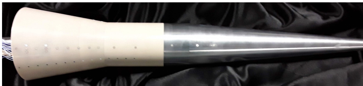
Figure 5.1. 10° cone-cylinder-flare model instrumented with PCB and Kulite pressure sensors, nosetip removed.
