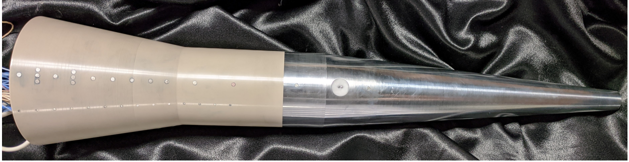
(a) 10° cone-cylinder-flare model with perturber electrodes installed. Nostip removed. The center of the electrodes is 387 mm downstream of the nostip, 12.7 mm from the expansion corner.
