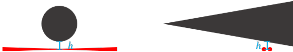
Figure 3.23. Illustration of FLDI beam placement relative to model, showing height off the surface, h . Not to scale.
