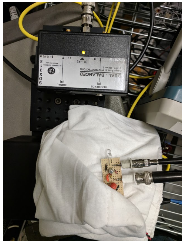
(b) Setup of LED test with photoreceiver and circuit
