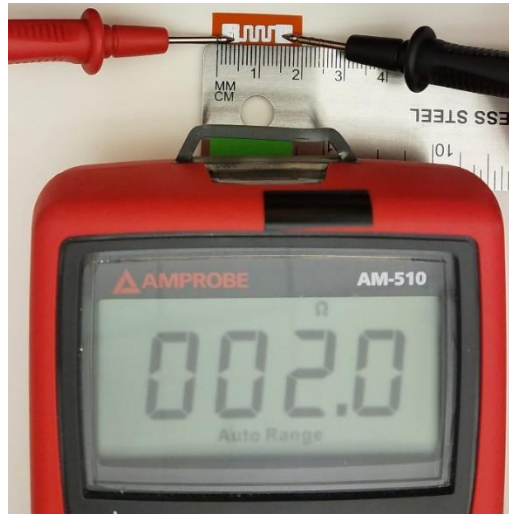
Figure A. 5. Low resistance microheaters are possible to create using the technique described in the main text. The design here has fewer serpentine turns resulting in a shorter path length. Specs: trace width: 0.529mm, path length: 24.264 mm, total heating area: 4 mm x 8.8 mm.
