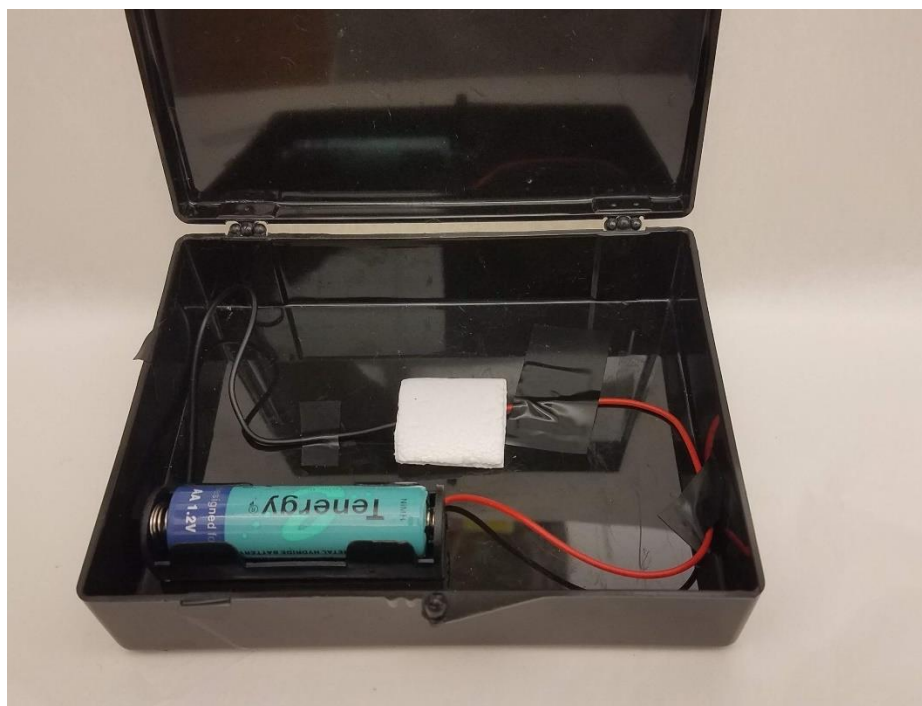
Figure C. 1. Setup for incubations powered by AA battery. Temperature sensors were placed on the top and bottom surfaces of the sample chip and the box was closed after initiation.
