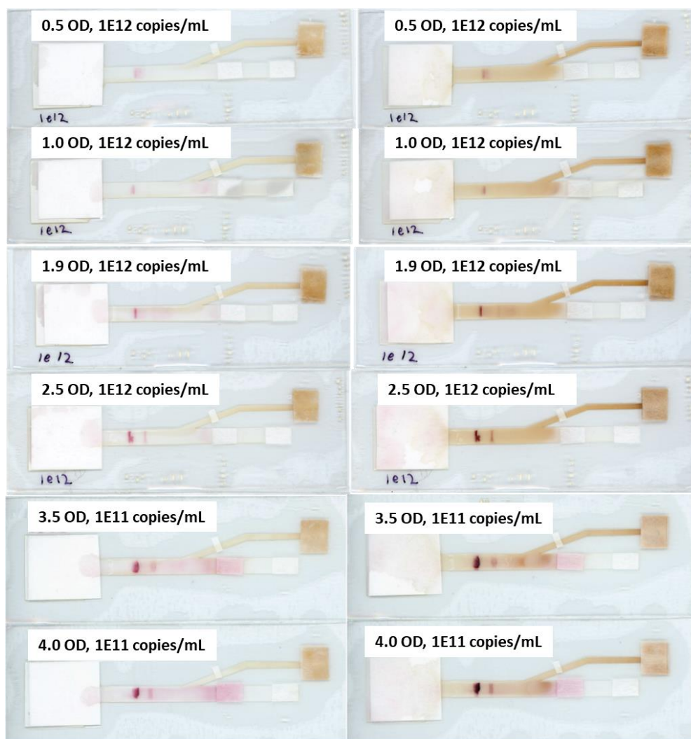
Figure 6.2 Representative samples from conjugated SA-HRP-AuNP Optimization. 20 minutes after flow initiation (left), 60 minutes after flow initiation (right). Other controlled variables: 1.4 mg/mL DAB and dried H 2 O 2 salt. .
