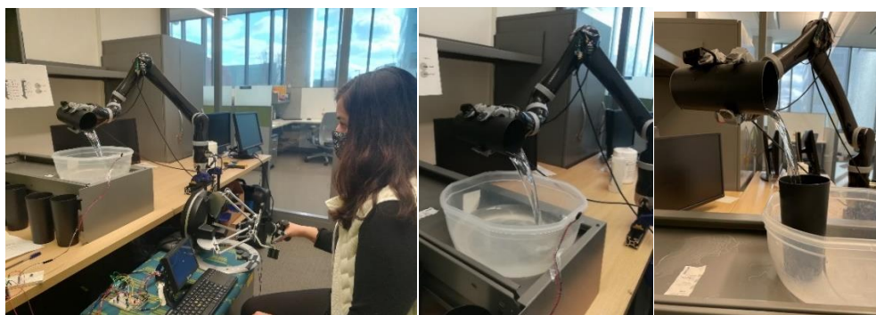
Figure 4.2: Experimental set-up for robot-assisted pouring task 01 (left), task 02 (center), and task 03 (right).
