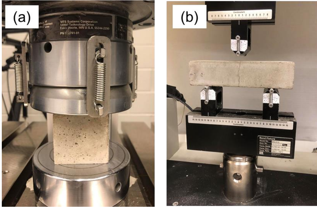
Figure 7: Experimental setup used for determination of (a) compressive strength and (b) flexural strength.
