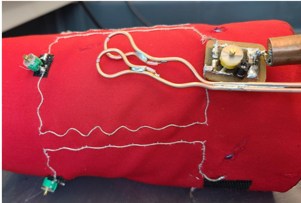
Figure 2.14 S_{21} measurement with an overlapped double-loop probe on a dielectric muscle phantom
