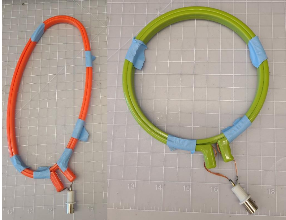
Figure 2.4 Oval (left) and circle (right) frames used for the impedance measurements
