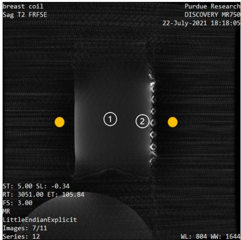
Figure 2.23 Regions of noise (yellow) and regions of signal (numbered) used for the SNR calculation in the sagittal T2 image. Signal region 1 is the center of the phantom, 2 is the center of the coil near the surface of the phantom.
