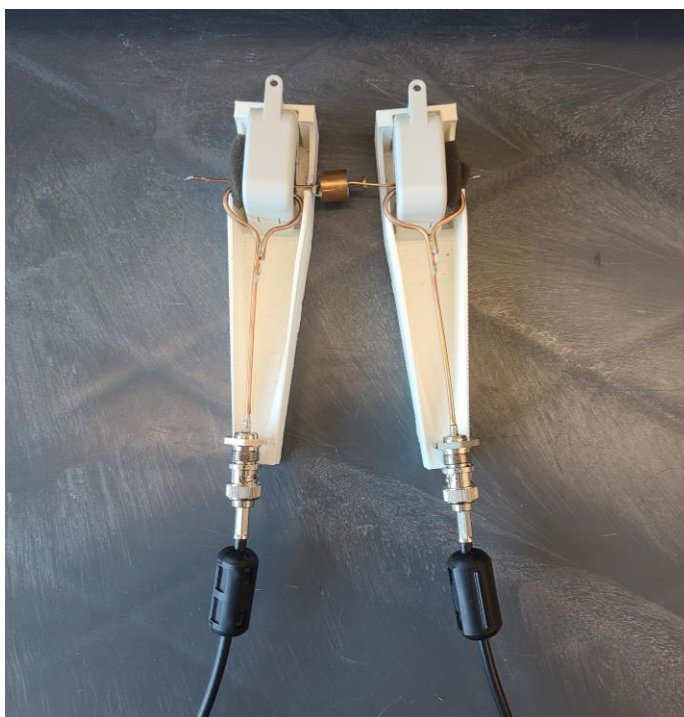
Figure 2.7 Bench setup of the S_{21} measurement for tuning a balun
