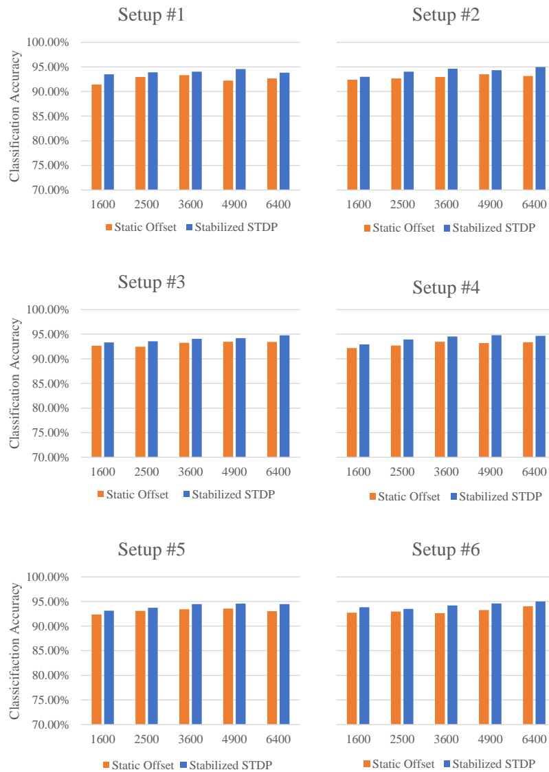
Figure 3.2. Unsupervised classification accuracy on MNIST using one-sided STDP with a static offset compared to stabilized on-sided STDP.
